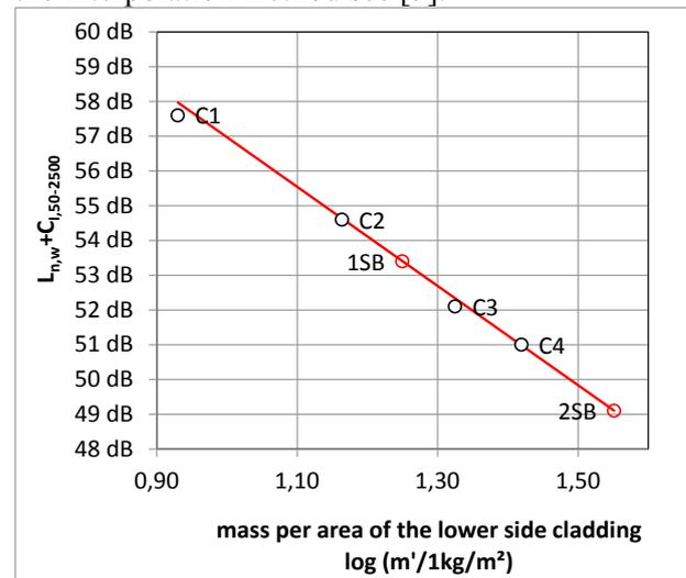
Figure 4: Interpolation of  $L_{n,w}+C_{1,50-2500}$ .
