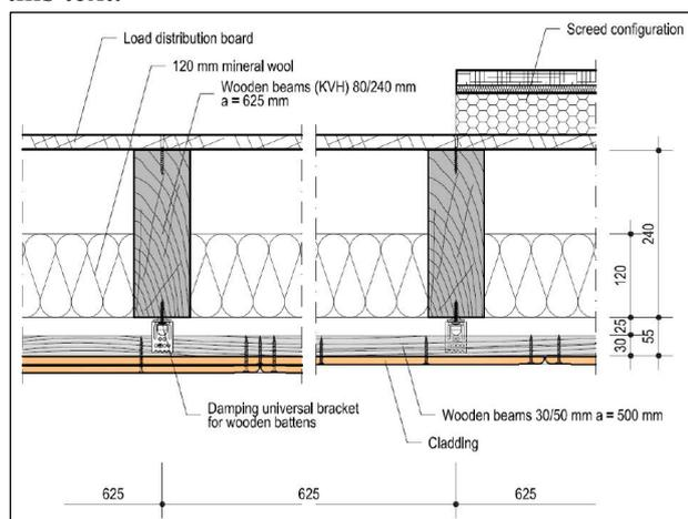
Figure 1: Basic ceiling, cross section perpendicular to the joists. Screed and lower claddings shown are examples.
