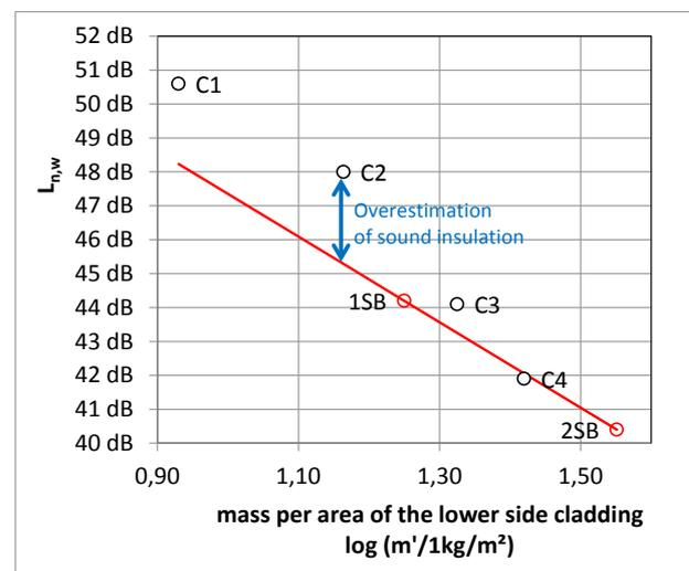
Figure 5: Interpolation of  $L_{n,w}$ . The straight line from measurement 1SB to measurement 2SB predicts a  $L_{n,w}$  up to 3 dB below the measured value.
