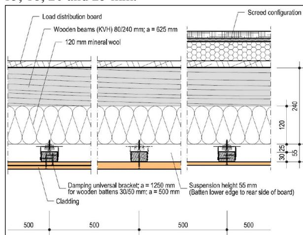
Figure 2: Basic ceiling, cross section parallel to the joists. Screed and lower claddings shown are examples.
