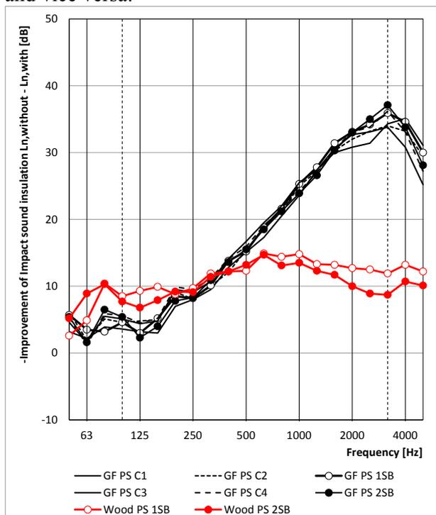
Figure 6: Improvement of screed PS on basic ceiling GF and Wood (Impact sound insulation).
