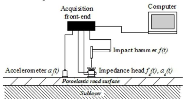
Figure 9. Experimental set-up for the determination of the mechanical impedance in situ (taken from [5])
