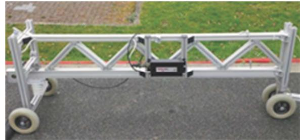
Figure 3. Static laser profilometer.
