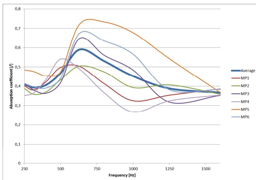
Figure 8. Third octave band results for the in situ measurements in Sterrebeek (MP = measuring point)
