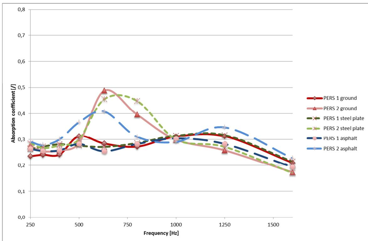
Figure 6. Third octave band results for two PERS test slabs
