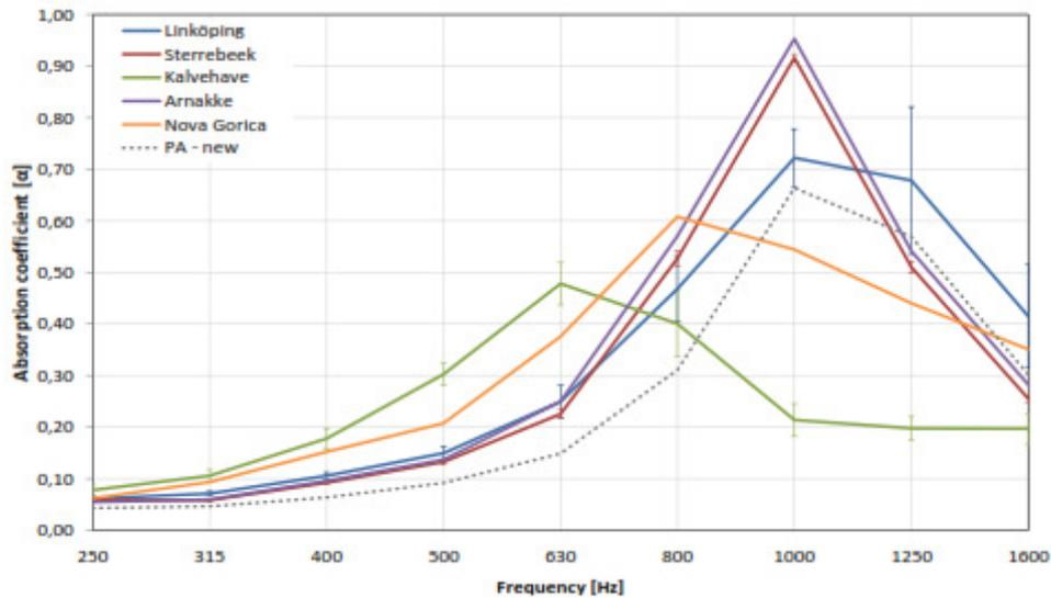
Figure 7. Third octave band results for cylindrical samples drilled from the different test sites in the PERSUADE project (taken from [5])
