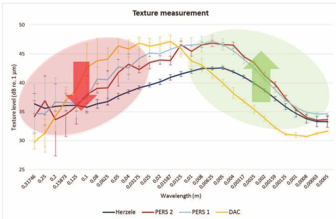
Figure 4. Comparison of the texture levels determined by laser profilometry on the PERS test sections and one dense asphalt concrete section (DAC)
