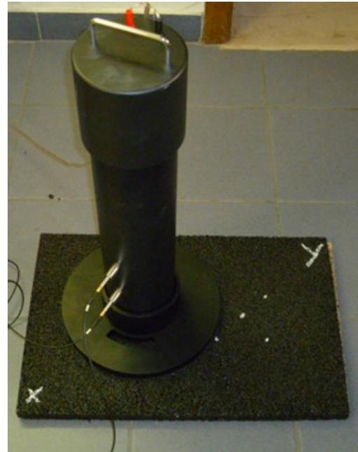
Figure 5. a BSWA-tech SW420R impedance tube
