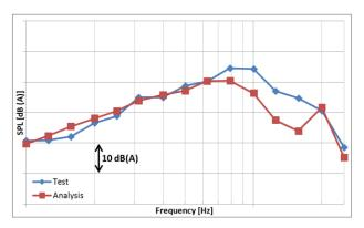
Figure 6. Rear region of front right tire to left ear of rear passenger.
