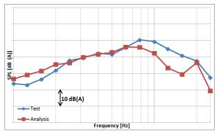
Figure 9. Front region of rear left tire to right ear of rear passenger.
