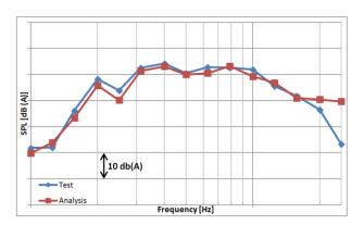
Figure 10. Rear region of front right tire to right ear of driver.
