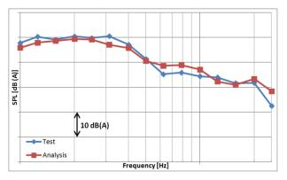
Figure 16. Response at right ear of driver @40 kph.
