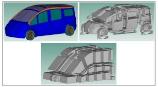
Figure 2. SEA subsystems of the vehicle
