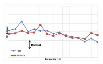
Figure 14. Response at right ear of driver @10 kph.
