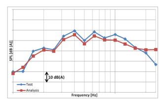
Figure 11. Rear region of front left tire to left ear of driver.
