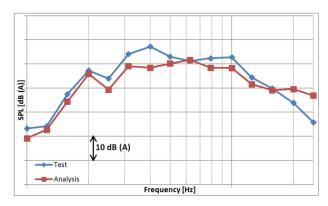
Figure 12. Front region of rear right tire to left ear of rear passenger.
