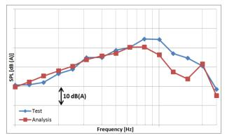
Figure 7. Rear region of front left tire to left ear of rear passenger.
