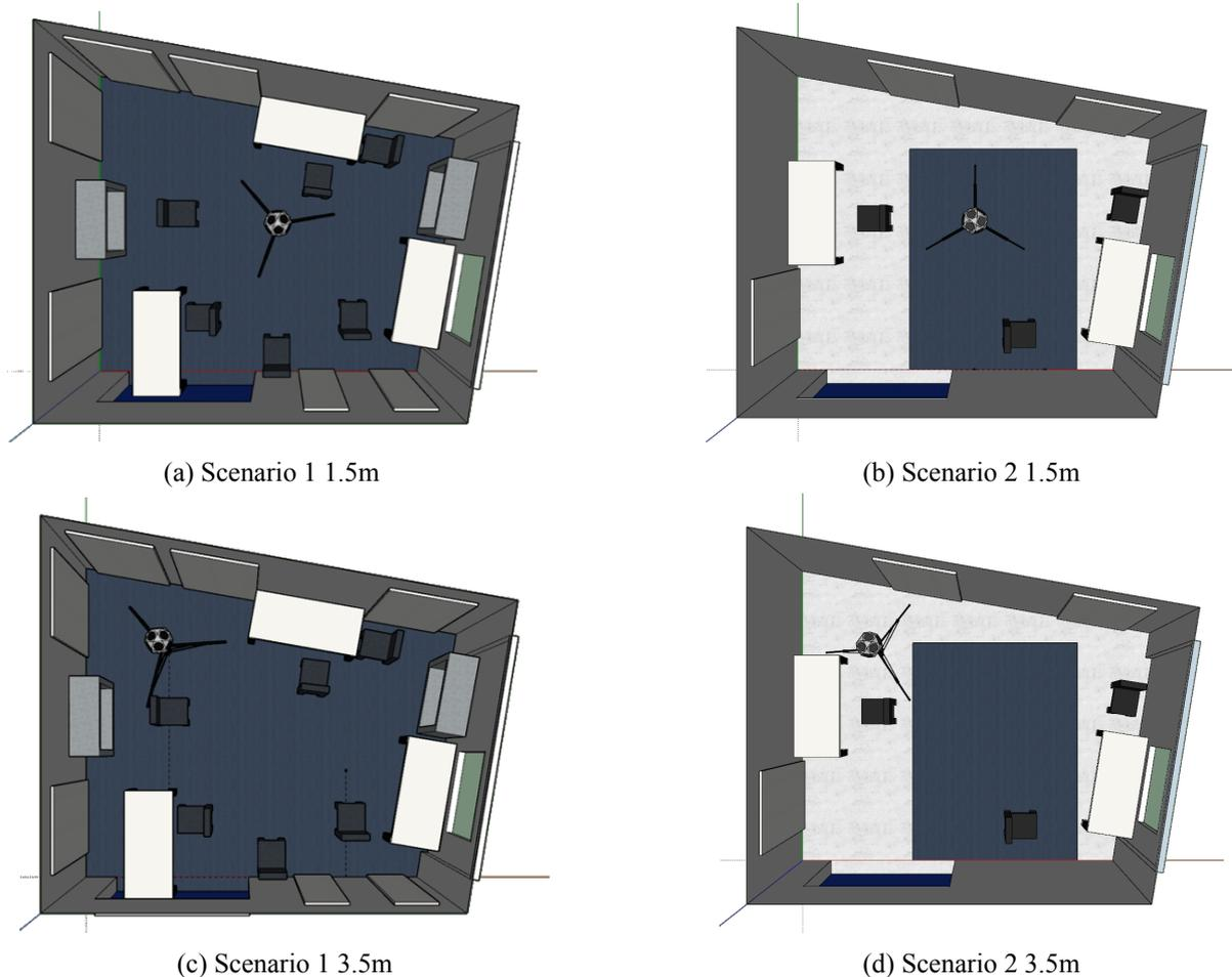
Figure 2: 3D room models of four room acoustic scenarios created in SketchUp.
