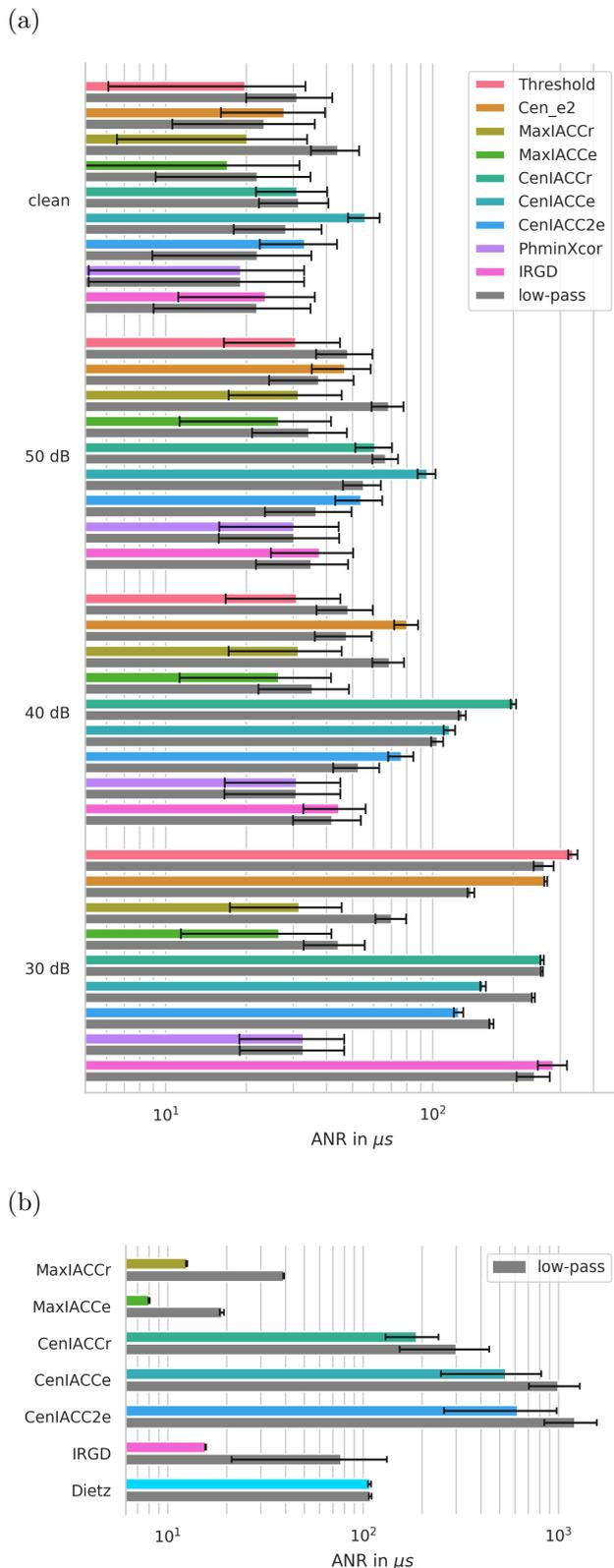
**Figure 3:** ANR of different ITD estimation methods (a) at different SNRs and (b) when applied to noise stimuli. The colored bars represent the ANR of the respective estimator based on broadband HRIRs. Error bars denote the standard errors of the means (across ear positions).
