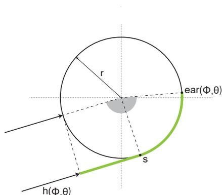
**Figure 2:** Illustration of the geometric model used to calculate TOAs. The circle represents the head with radius  $r$ . The green line shows the propagation path of the incoming wave  $h(\Phi, \theta)$  to the ear position  $\text{ear}(\Phi, \theta)$  used to calculate the TOA.
