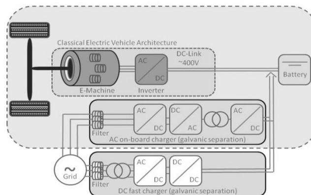
Figure 1: Schematic view of on-board charger and electric vehicle architecture (extracted from [2]).
