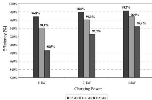
Figure 4: Calculated efficiency of on-board constant switching frequency charger (extracted from [10]).
