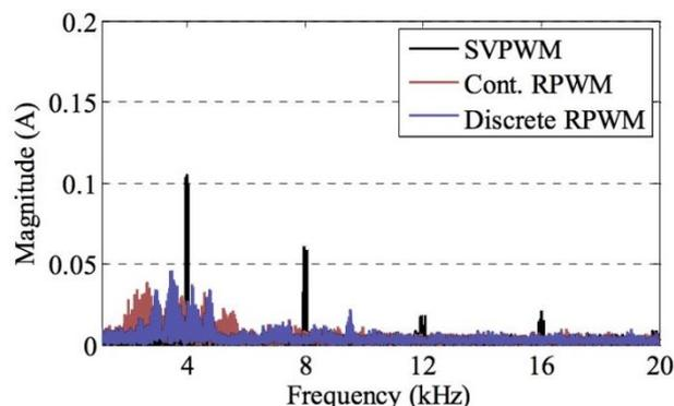
Figure 5: Comparison of current spectrum of single frequency PWM (SVPWM) and random PWM (RPWM) – extracted from [12].
