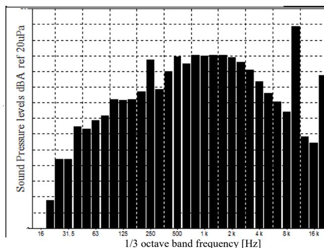
Figure 6: Sound pressure levels at 1m during  $>20$  kW charging of commercial BEV.
