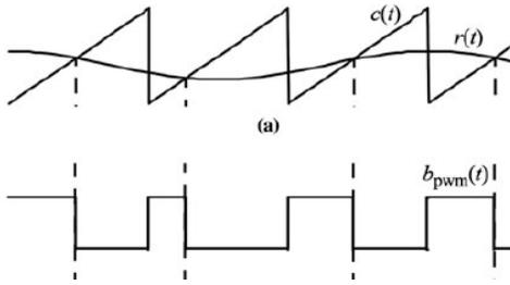
Figure 2: Pulse width modulation of constant frequency trailing edge saw tooth carrier (extracted from[5]).
