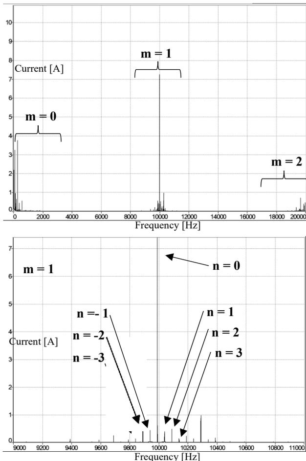
Figure 3: Example of the DC-side current spectrum of a 22 kW charger up to 20 kHz and zoomed around the carrier wave frequency 10 kHz. The harmonic currents are concentrated around  $m = 0, 1$  and  $2$ .
