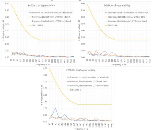
Figure 9 : Impact of the type of excitation on  $\sigma$  of repeatability in the three test facility Vs ISO 12999-1 one
