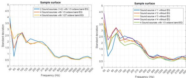
Figure 6: Standard deviation of the Lp at 5 cm of the test sample
