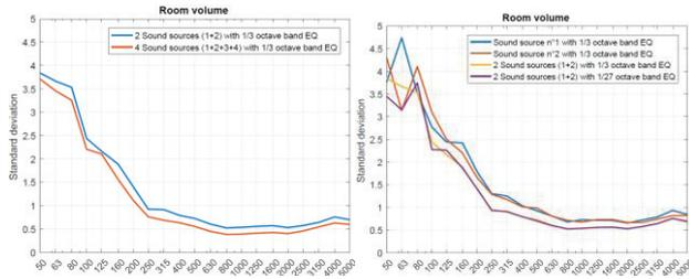
Figure 5: Standard déviation between Lp in the volume, for different type of excitation (both) and for different equalization (right - yellow and purple curves)
