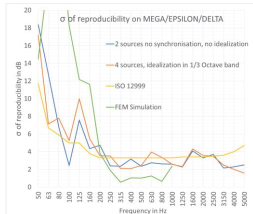
Figure 11 :  $\sigma$  of reproducibility on three facilities, comparison of measured and simulated one.
