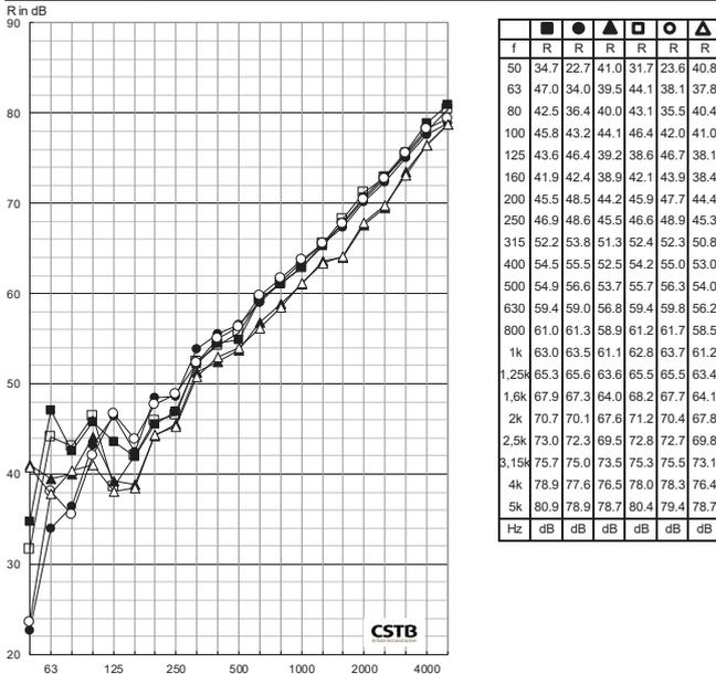
Figure 8 : Airborne sound insulation in the three facilities with two type of excitation
