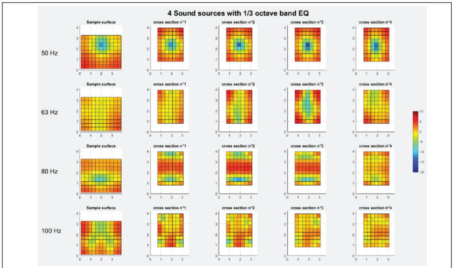
Figure 12 : Exemple of the sound field scanning in between 50Hz and 100Hz - 4 sources equalized in 1/3 octave band
