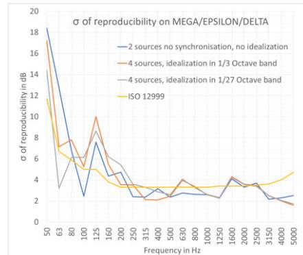
Figure 10 :  $\sigma$  of reproducibility on three facilities, for three excitation compare to ISO 12999-1 curve.
