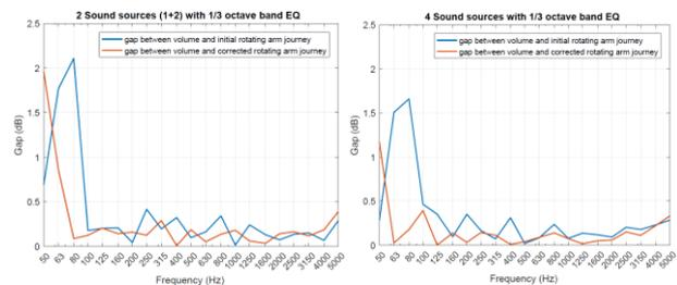
Figure 3: Difference between  $L_p$  averaged on the volume and  $L_p$  averaged on the rotating boom (For two type of excitation and two position of rotating boom).
