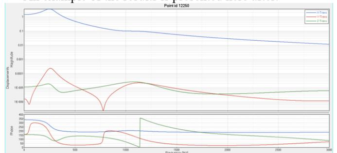
Figure 13 : Example of dynamic stiffnesses of the mounts
