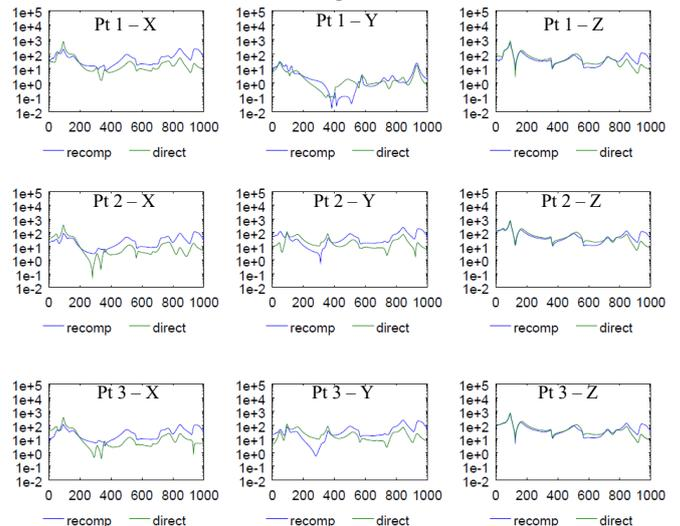
Figure 18 : Comparison between recomposed forces (---) and direct calculation forces (---)
