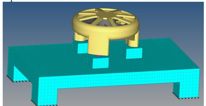
Figure 6 : Meshed fan unit with elastomeric mounts on the bench
