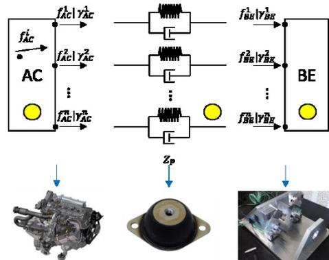
Figure 2 : Active component and mounts on the bench – ○ characterized by tests
