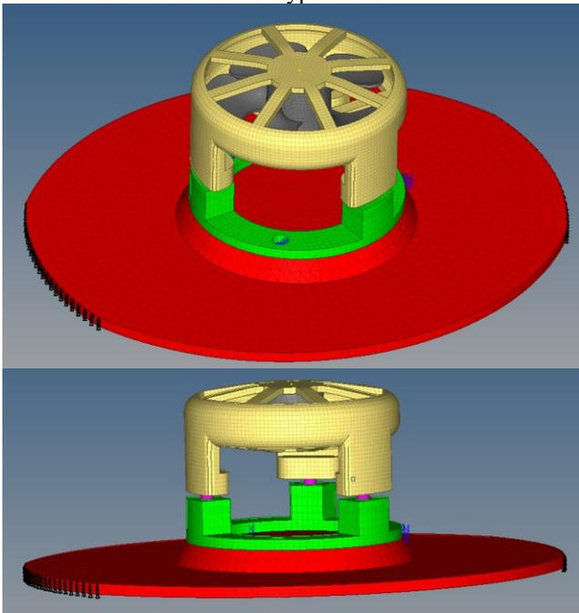
Figure 3 : Meshed fan unit on reception component with interface and elastomeric mounts
