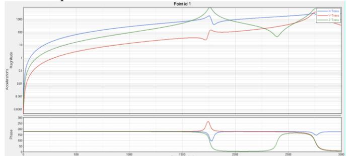
Figure 5 : Example of inertances and cross-transfers on the bench
