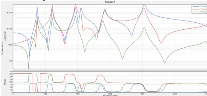
Figure 15 : Example of inertances and cross-transfers on the interface
