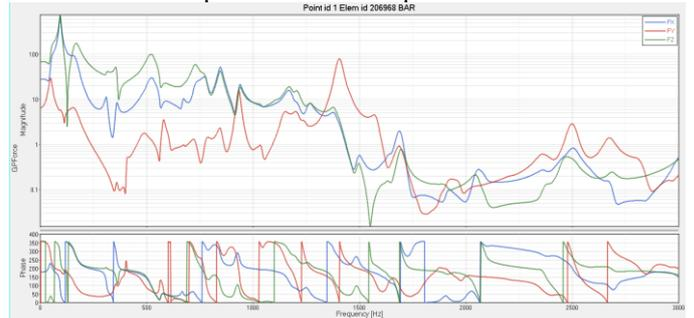
Figure 17 : Example of measured forces injected to the passive component
