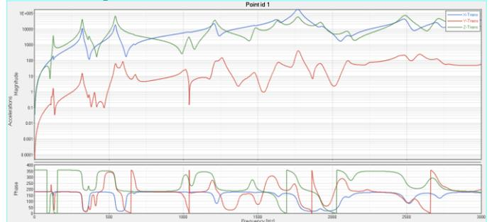
Figure 11 : Example of inertances and cross-transfers on the bench
