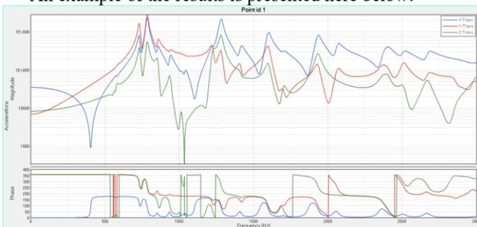
Figure 9 : Example of inertances and cross-transfers on the active component
