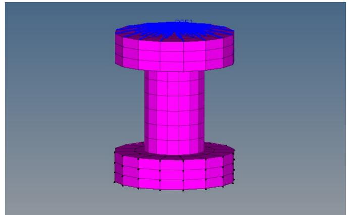
Figure 12 : Meshed fan elastomeric mounts
