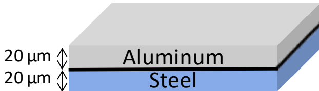
Figure 3: Isotropic multilayered structure with an imperfect interface.
