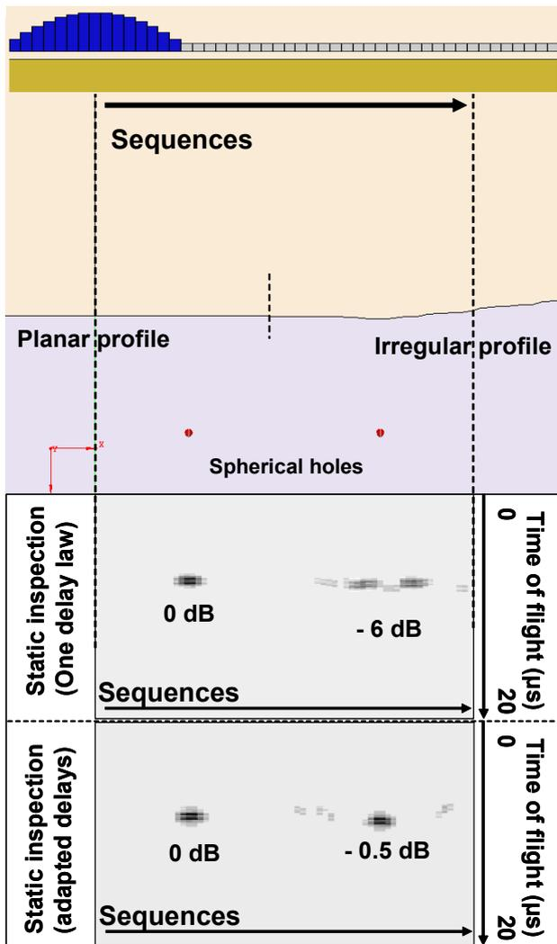
Figure 5: Electronic commutation with a linear array over a planar and complex profile. Inspection simulation using a static mode and a dynamic mode.
