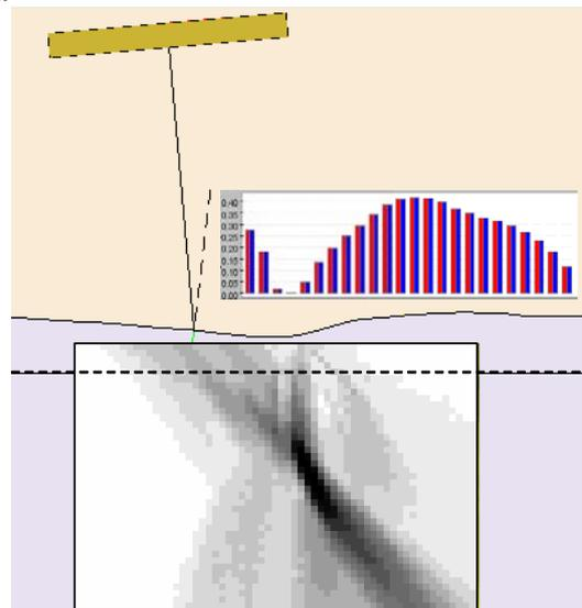
Figure 4 : Field radiated through the anisotropic/isotropic and irregular profile using adapted delay laws
