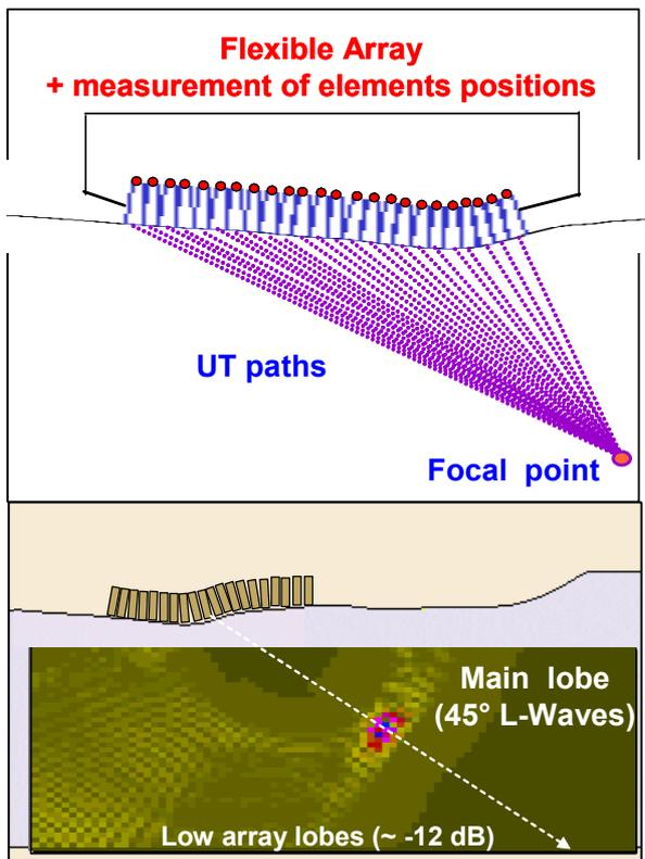
Figure 6: Principle and example of transient beam computation of a flexible array probe
