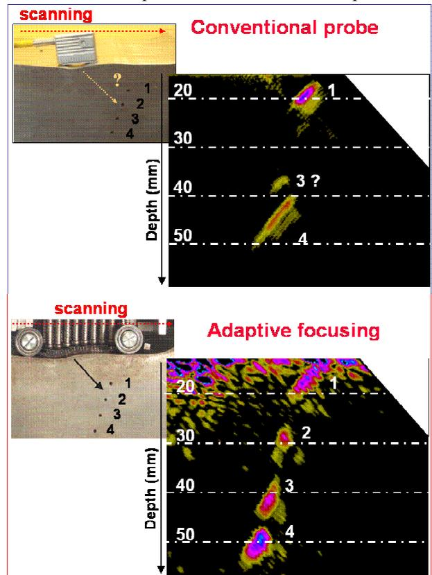
Figure 7: Inspection of a complex profile specimen with a standard contact probe (top) and the flexible array probe (bottom) using 45° shear waves
