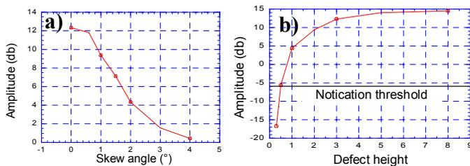
Figure 2: Demonstration performance of the inspection of the upper shell of steam generator of PWR. Influence of a) the skew angle, and b) the defect size.
