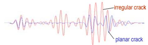
Figure 7: The hybrid model: Comparison between the computed Ascan issued from the irregular and planar cracks
