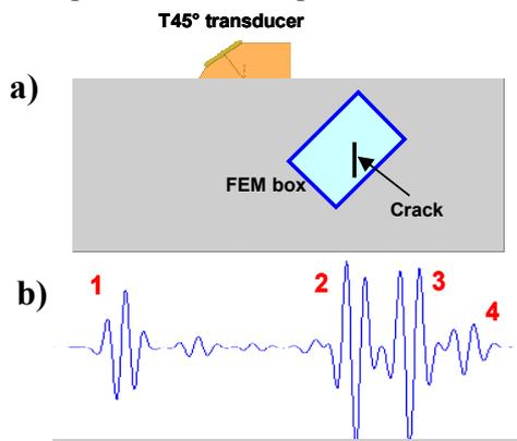
Figure 6: The hybrid model: Computation of the response of a planar crack. a) simulated configuration; b) computed Ascan
