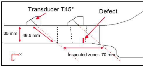
Figure 1: Demonstration performance of the inspection of the upper shell of steam generator of PWR. Zoom on the inspected area
