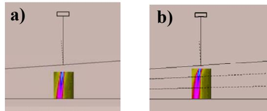
Figure 4: Simulation of the inspection of the component of Figure 2a). Computed beams a) without taking into account the varying orientation of plies; b) taking it into account.
