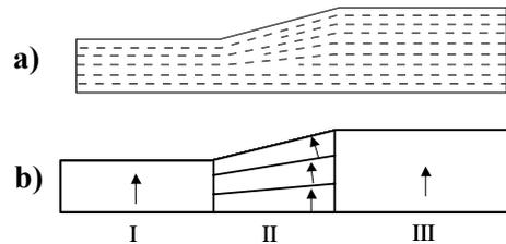
Figure 3: Homogenization of a multi-layered composites. Schematized view of a) the component (dotted lines indicating the orientation of plies) and b) the homogenized description.
