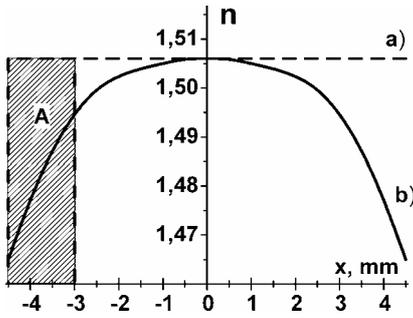
Figure 7 : Refractive index distribution along  $x$ -axis for samples: a) for glass preform, b) for gradient waveguide.  $x = 0$  corresponds to  $\nabla \bar{n}$  direction change, A – gradient area of the sample
