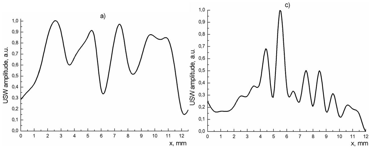
Figure 4 : Amplitude distribution of longitudinal USW on butt-ends of the samples in direction  $x$ :
