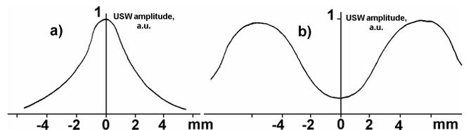
Figure 6 : Distributions of amplitude of longitudinal pulse USW with frequency 14 MHz at an end face: a) of the gradient glass cylinder with «focusing» distribution of elastic properties (fig. 9), b) of the homogeneous glass cylinder (of the same sizes)
