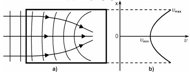
Figure 1 : a) Schematic of USW propagation in gradient acoustic (or optical) waveguide, b) distribution of velocity of longitudinal USW (or velocity of light) in the waveguide
