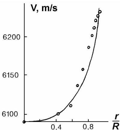
Figure 5 : Actual distribution of longitudinal USW velocities in the gradient glass cylinder (circles) and calculated by (1).  $R$  – cylinder radius
