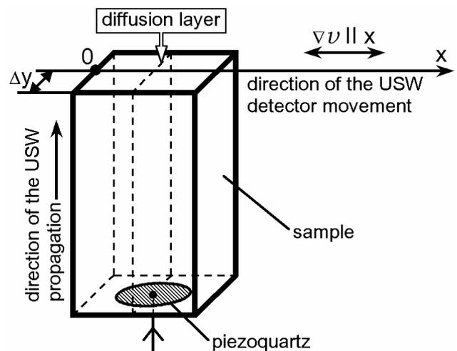
Figure 3 : Schematic of scanning the sample butt-end by the USW detector in two directions:  $\nabla v \parallel x$  or  $\nabla v \perp x$ .  $\nabla v$  - elastic properties gradient direction,  $\Delta y$  - shifting of USW detector concerning the sample butt-end edge
