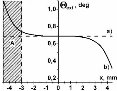
Figure 8 : External Bragg angle  $\Theta_{\text{ext}}$  versus  $x$ -coordinate of beam entrance into samples: a) for glass preform, b) for gradient waveguide (A – gradient area of the sample).  $\nu = 210$  MHz,  $v = 5600$  m/s,  $\lambda_0 = 632,8$  nm
