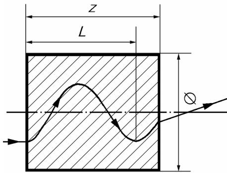
Figure 2 : Schematic of propagation of acoustical ray in the gradient cylinder with «focusing» distribution of elastic properties according to (1)
