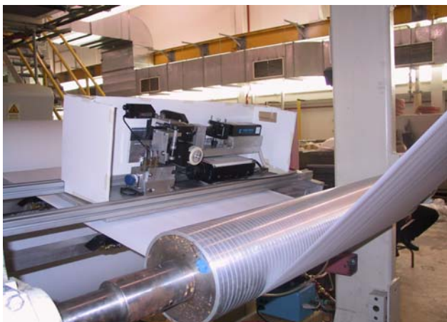
Figure 1. LUS system installed on pilot coating machine.
