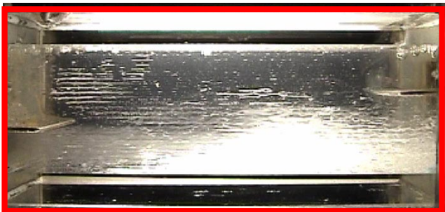
Fig.8. Frame picture of the h-separator performance. The output flow ratio V_{O1} / V_{O2} = 1 corresponds to a respective ratio of the mean flow velocities of 2:1, because the cross sectional area of output O1 was chosen half the value of the cross sectional area of output O2.
