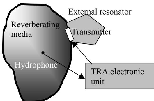
Figure 1. The concept of TRA focusing reverberation media with an external resonator
