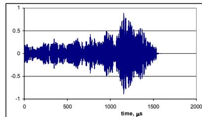
Figure 8. Time tracks for TRA focusing of the amplitude modulated r.f. pulse:
