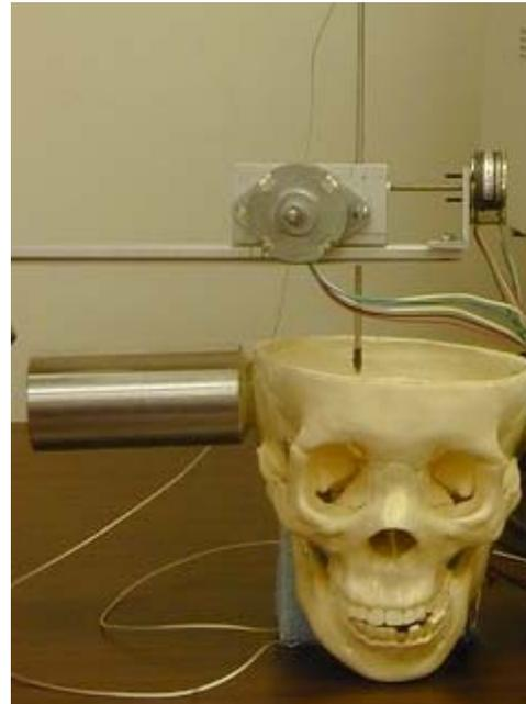
Figure 4. Skull model with an external aluminum resonator and a hydrophone mounted on a 3-D positioning system to map generated acoustic fields
