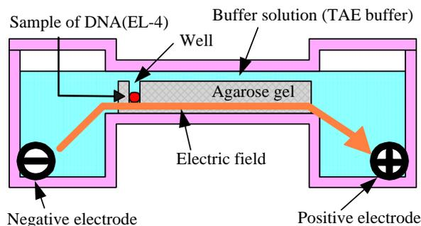
Fig. 4 Apparatus for agarose gel electrophoresis
