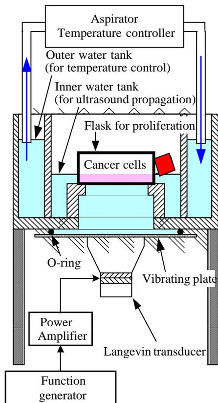
Fig.3 Basic structure of ultrasound exposure system for suppression of cancer cells proliferation
