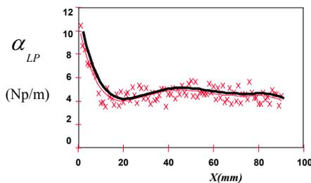
Fig.5 longitudinal wave attenuation coefficient on the axis
