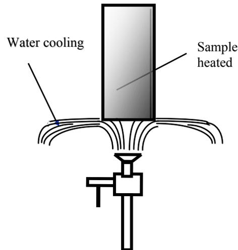
Fig.3 heat treatment device
