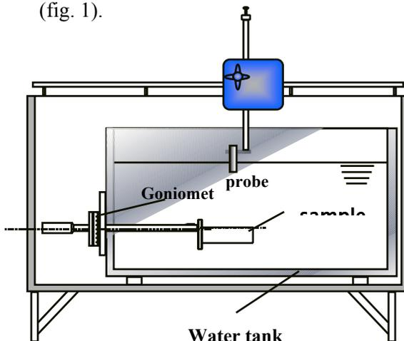
Fig.1. experimental device
