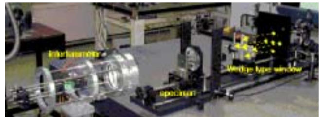
Figure 2 : Experimental arrangement from beam split unit (multi-beam irradiation module) to interferometer
