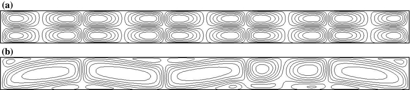
Figure 3: Streamlines for  $Re = 300$ . (a) classical Rayleigh streaming. (b) asymmetric flow.
