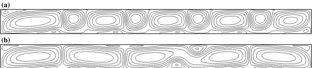
Figure 5: Streamlines for  $Re = 700$ . Different type asymmetric flows.
