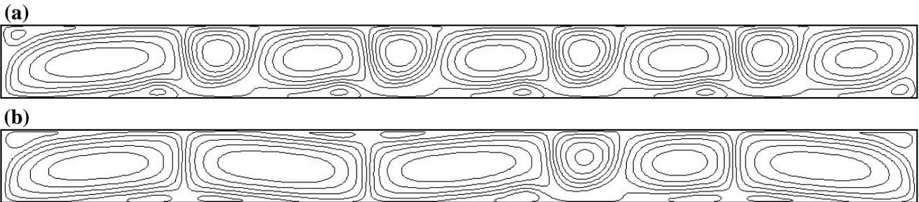
Figure 4: Streamlines for  $Re = 600$ . Different type symmetric flows.
