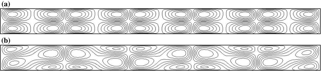
Figure 2: Streamlines for  $Re = 140$ . (a) classical Rayleigh streaming. (b) symmetric flow.
