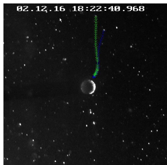
Figure 3: Images of particles and particle trajectories obtained from the experimental chamber.
