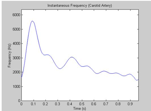
Figure 4 : Theoretical  $PIMF$  of the simulated ultrasonic Doppler signal.
