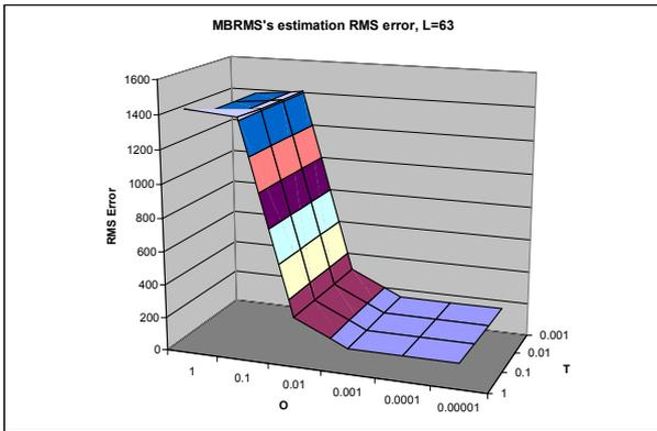
Figure 3 : RMS error function of the  $MB_{RMS}$  estimation with a sampling window length of  $L = 63$ .
