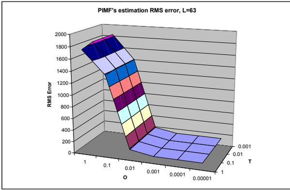
Figure 2 : RMS error function of the PIMF estimation with a sampling window length of  $L = 63$ .
