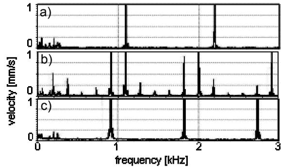
Figures 3a, b, c: Interchangeable generation of subharmonics (a, c) and frequency pairs (b) by a crack in a polystyrene plate.
