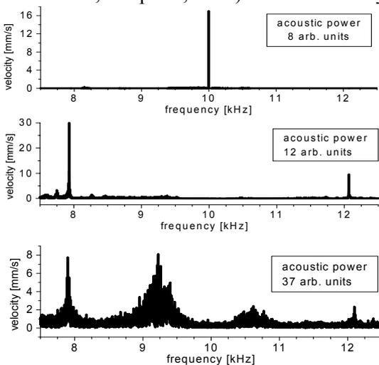
Figure 2: Subharmonic-frequency pairs-frequency bands series in a delamination area in C/SiC ceramic sample.
