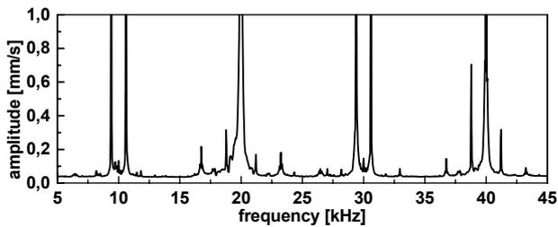
Figure 8: Self-modulation spectrum for the sample of a epoxy-based textile composite with an impact. Excitation frequency is 20 kHz.
