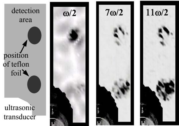
Figure 6: Subharmonic images of simulated delamination area in a Glare® sample
