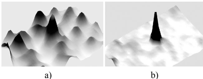
Figures 9a, b: Self-modulation imaging of an impact in GFR-composite: a) 4<sup>th</sup> harmonic image; b) self-modulation (side-lobe of the 10<sup>th</sup> harmonic) image.
