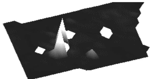
Figure 7: Subharmonic image of cracked area in FR-ceramic. Excitation frequency  $\approx 27$  kHz corresponds to one of the resonance frequencies of the defect.
