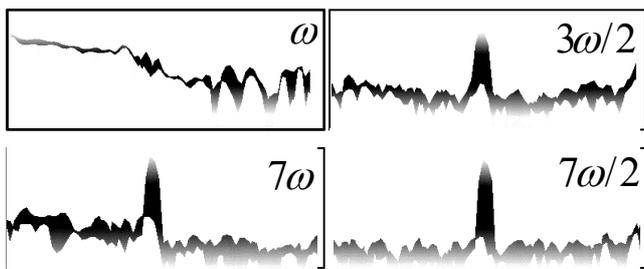
Figure 5: Linear, higher harmonic and subharmonic images (B-scans) of a knot in the middle of a 50 cm-long wooden rod. Vibrations are excited at the left-hand side edge of the specimen.
