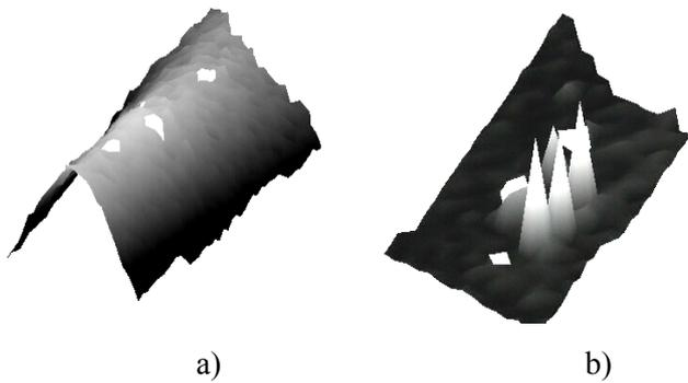
Figures 1a, b: Vibration patterns of cracked FR-ceramic sample: a) bending mode sample resonance (1350 Hz); b) one of the resonance modes of cracked area ( $\approx 81$  kHz). The holes (seen in the picture) are made to initiate cracking.
