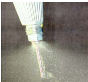
Figure 6 : Atomization and source of “hiss” from shoulder of tip.
