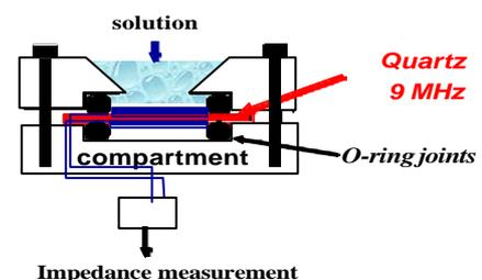
Figure 1 : Scheme of the experimental device.
