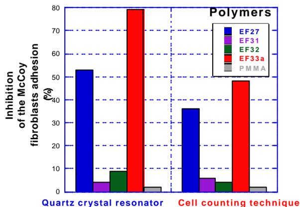
Figure 5: Comparison of cell adhesion by the quartz crystal resonator and cell counting techniques.
