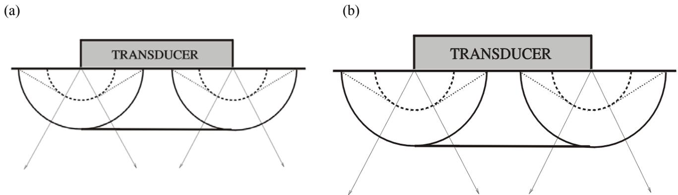
Figure 3: The wave fronts in geometrical zones (a) and transition zones (b) underneath a circular transducer acting normally to the surface of a half-space. Solid line - P fronts, dashed line - S front. Light-shaded area - penumbra (Fresnel's function), dark-shaded area - the axial zone (Bessel's functions). The arrows indicate the wave polarization. The conical head wave front is not indicated.
