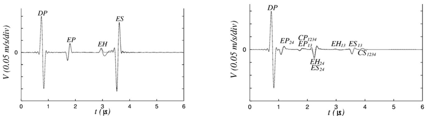
Figure 4: Typical waveforms of the particle velocity at the  $e_3$  - axis of a (a) circular and (b) rectangular transducer. Solid and dashed lines are the exact and asymptotic solutions respectively. DP - the direct P wave, EP, ES or EH - the edge P, S or head wave from the point  $E_i$  and  $CP_i$ ,  $CS_i$  or  $CH_i$  - the corner P, S or head wave from the point  $C_i$ .
