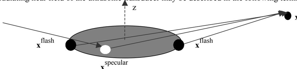
Figure 2: A typical observation point  $x$  and specular and flash points  $x^{\text{specular}}$  and  $x^{\text{flash}}$  on a circular transducer.
