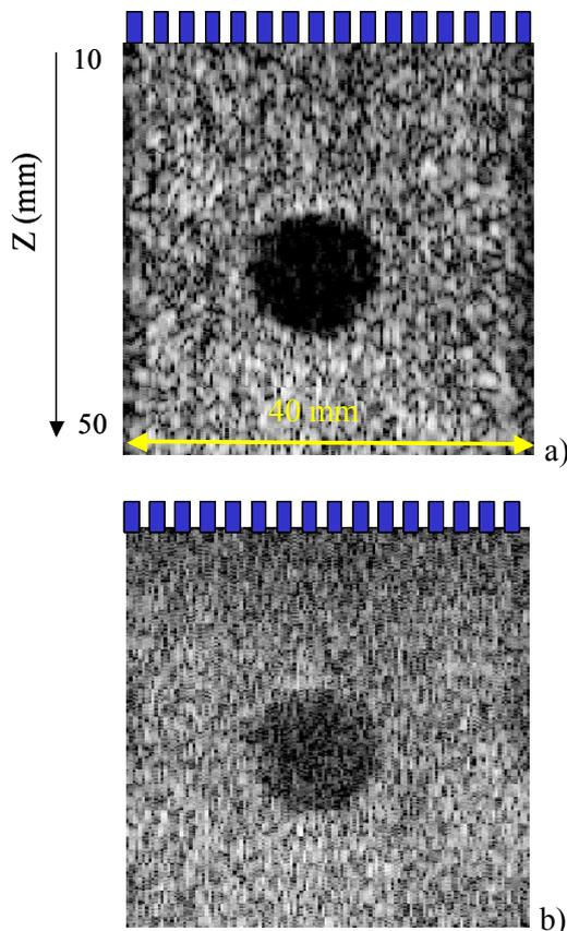
Fig. 6. a) fundamental and b) harmonic image of an Agar gelatin phantom presenting an anechoic inclusion. The contrast in the harmonic image is quite low. M.I. was equal to 1. The probe is working at 4.3 MHz.
