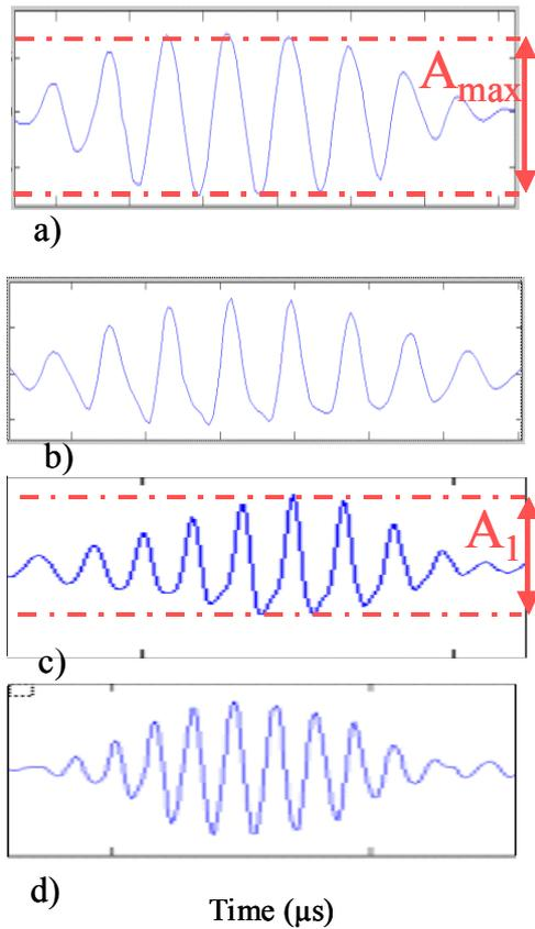
Fig. 3. Experimental results : a) signal emitted by the array; b) backscattered echo after nonlinear propagation in water; c) time reversal and transducer bandwidth correction of the received echo; d) backscattered echo after reemission of the signal presented in Fig. 3.c.
