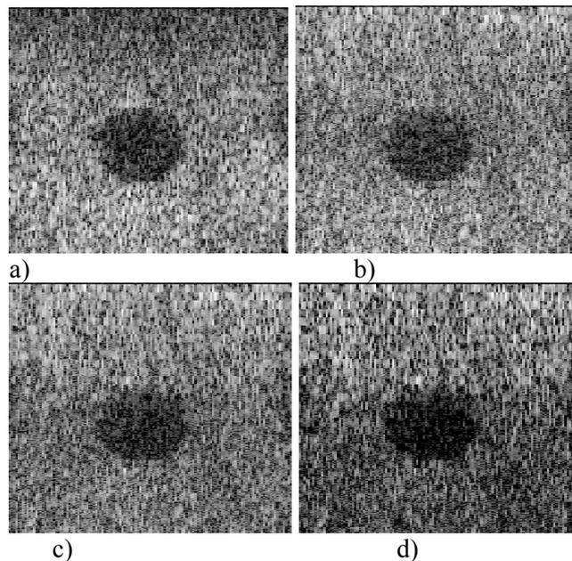
Fig. 8. Experimental harmonic images obtained using distorted emission waveforms. The harmonic content of the agar gelatin phantom surrounding the anechoic inclusion is progressively cancelled.
