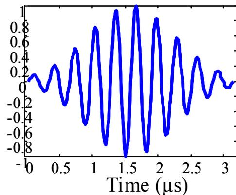
Fig. 5. Conventional emission signal used for the beamforming process of the fundamental and harmonic images of the experimental Agar gelatin phantom presented in Fig. 6.
