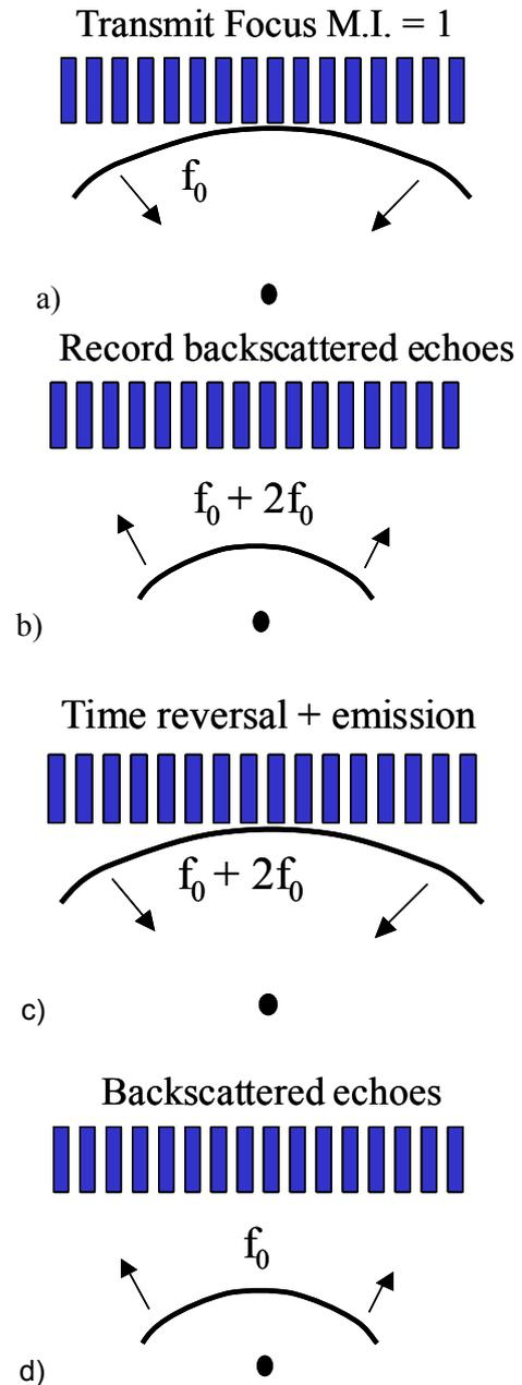
Fig. 2. Principle of the adaptive cancellation of harmonics due to nonlinear propagation.
