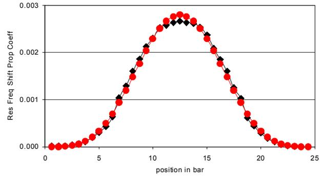
Fig.2: Sensitivity of the resonance frequency-shift to the damage location of the first mode. Circles (theory:  $\sin^4$ -fit of Eq.(17))-Diamonds (Simulation).
