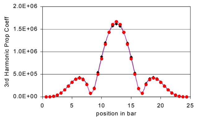
Fig.3: Sensitivity of the third harmonic amplitude to the location of the damage. Circles (theory: Fit according to Eq. (19))-Diamonds (Simulation).
