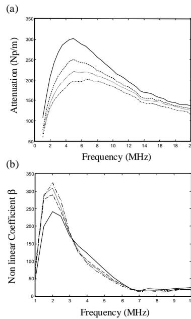
Figure 6: Measured (a) attenuation and (b) nonlinear coefficient in SonoVue<sup>®</sup> solution with an initial volume fraction  $z = 4.5 \cdot 10^{-6}$ , at times  $t_1=0$  (solid line),  $t_2=15$  min (dashed line),  $t_3=30$  min (dotted line), and  $t_3=45$  min (dash-dotted line) after bubbles injection.
