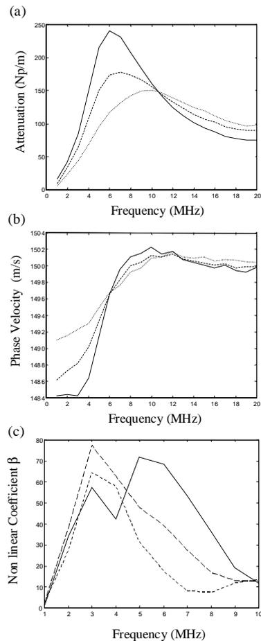
Figure 5: Measured (a) attenuation, (b) phase velocity and (c) nonlinear coefficient in Sonazoid<sup>®</sup> solution with an initial volume fraction  $z = 9 \cdot 10^{-6}$ , at times  $t_1=0$  (solid line),  $t_2=15$  min (dashed line), and  $t_3=30$  min (dotted line) after bubbles injection.
