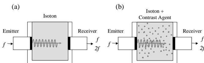
Figure 3 : Second harmonic insertion – substitution principle.
