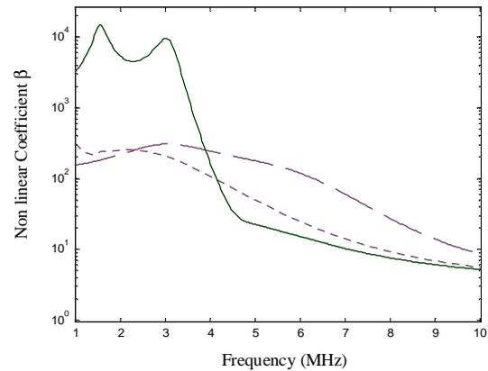
Figure 1 : Nonlinear coefficient vs. Frequency for a solution containing uniform radius  $R_0 = 1.2 \mu\text{m}$  free gas bubbles (solid line), uniform radius  $R_0 = 1.2 \mu\text{m}$  encapsulated Sonazoid<sup>®</sup> gas bubbles (dashed line), and a real radii distribution of Sonazoid<sup>®</sup> gas bubbles (dotted line) with a volume fraction  $z = 10^{-5}$ .
