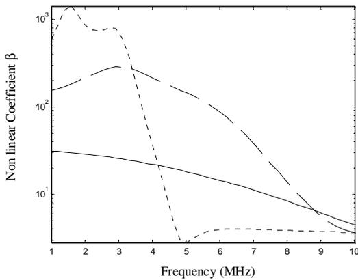
Figure 2 : Nonlinear coefficient vs. Frequency for a solution containing uniform radius encapsulated Sonazoid<sup>®</sup> gas bubbles, with  $R_0 = 0.5 \mu\text{m}$  (solid line),  $R_0 = 1.2 \mu\text{m}$  (dashed line) and  $R_0 = 2 \mu\text{m}$  (dotted line).
