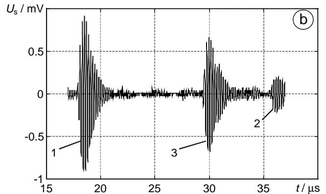
Figure 3: Ultrasonic waveforms of the waveguide type transducer with the GaPO<sub>4</sub> crystal: a - the first (1) and the second (2) reflections in the waveguide before immersion in the liquid Pb/Bi, (in air at 20°C); b – after the immersion into the liquid Pb/Bi at the temperature 250°C
