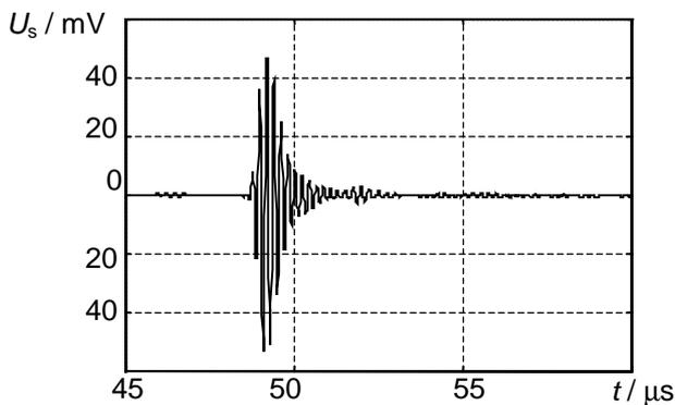
Figure 2: Pulse response of bismuth titanate Pz46 ultrasonic transducer with a thin ( $\lambda/2$ ) protector in the Pb/Bi alloy at 160°C
