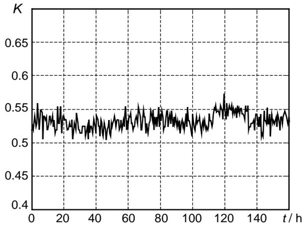
Figure 4: Time variation of the acoustic contact with the liquid Pb/Bi alloy at the temperature 200°C.
