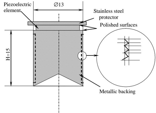
Figure 1: Monolithic transducer design with a metallic backing
