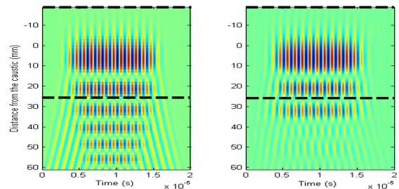
Figure 2 : Prescribed (left) and measured (right) linear field around the fold caustic
