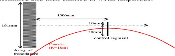
Figure 1 : Geometry of the experiment for the fold caustic
