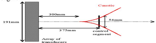
Figure 5 : Geometry of the experiment for the cusp caustic
