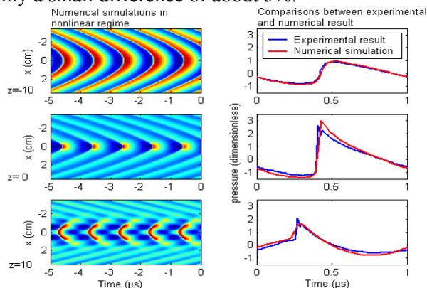
Figure 8 : Simulated fields at 3 distances from the cusp and comparisons on  $x=0$  between numerical simulations and measurements.
