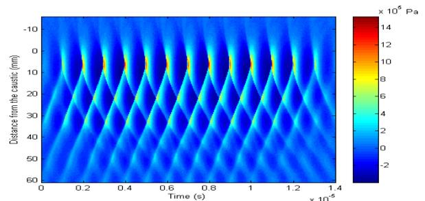
Figure 3 : Measured nonlinear field around the fold caustic
