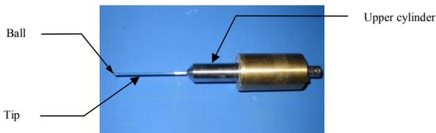
Figure 6: The sensor developed for microscopy is composed of a metal upper cylinder, a glass tip and a stainless steel ball.
