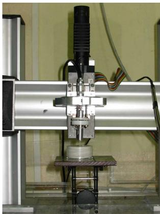
Figure 3: Experimental set-up : the tip of the sensor is dived in the analyzed medium.
