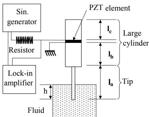
Figure 1 : Geometry of the sensor. The electric circuit is composed of a sinusoidal wave generator and a Lock In Amplifier
