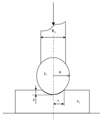
Figure 5: the ball glued at the end of the sensor is in contact with the flat surface of the sample.
