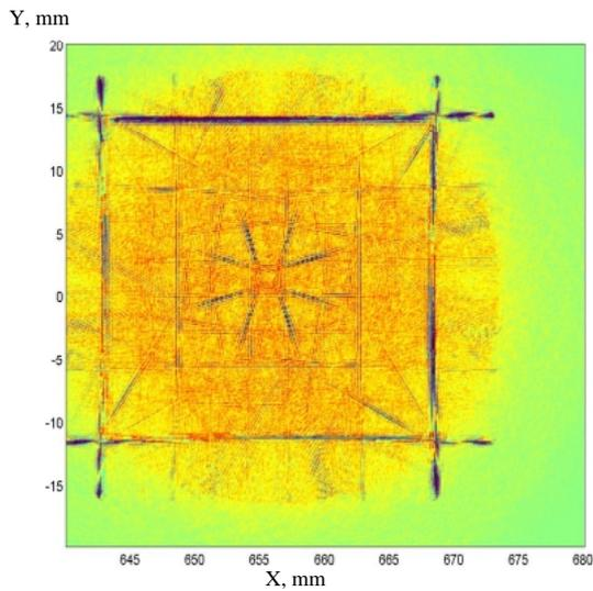
Figure 6: The reconstructed image of the rectangular bar obtained from the data with the 10dB gain
