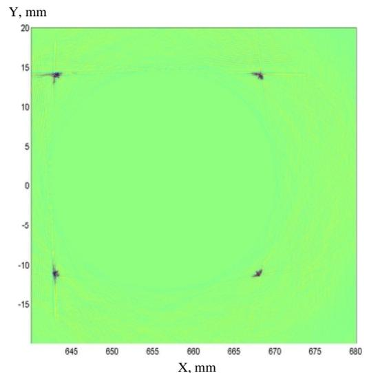
Figure 8: The reconstructed image of the rectangular bar obtained only from the edge wave signals. The four points correspond to position of edges objects in obtained images at the moment can be recognized only visually, because the object in the image is blurred and presented by dashed lines.
