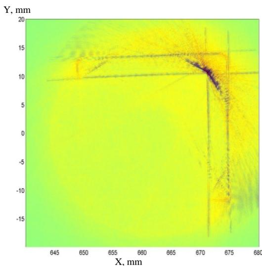
Figure 7: The reconstructed image of the L-shape profile obtained from the data with the 10dB gain
