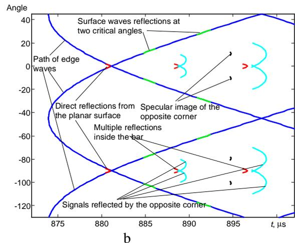
Figure 4: a - The normalised B-scan image of the rectangular bar in the case of the 50dB gain; b - distribution of different analysed signals in the time domain
