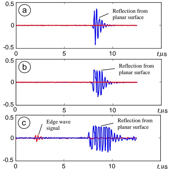
Figure 3: The signals reflected by the rectangular bar and collected using a different gain of amplifiers: a – 10dB, b – 30dB, c – 50dB
