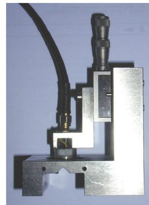
Figure 4 : A specific mechanical holder to fix the transducer to the rod.
