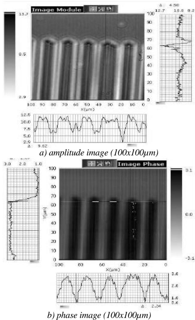
Figure 4: acoustic images and profile examples of the etched side of the PPLN device
