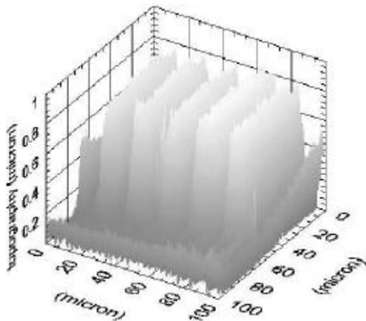
Figure 5: topography detected from acoustic phase measure at 600MHz
