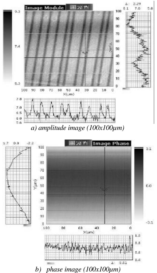
Figure 6: acoustic images and profile example of the virgin side of the PPLN device
