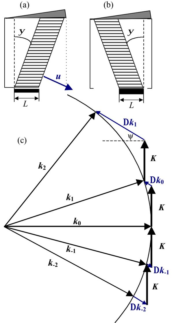
Figure 2: ULD in an elastically anisotropic medium at light incidence parallel to the sound wave fronts.
