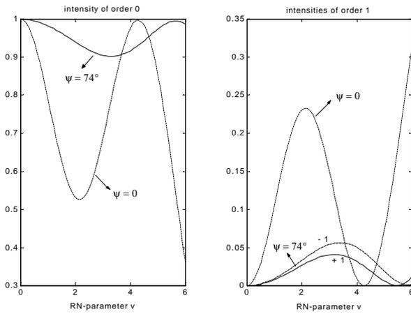
Figure 3: ULD at 20 MHz in TeO<sub>2</sub> in case of normal light incidence and  $\gamma = 74^\circ$ . Intensities of order 0 and  $\pm 1$  versus  $v$ . Dashed lines refer to the case  $\gamma = 0$ .
