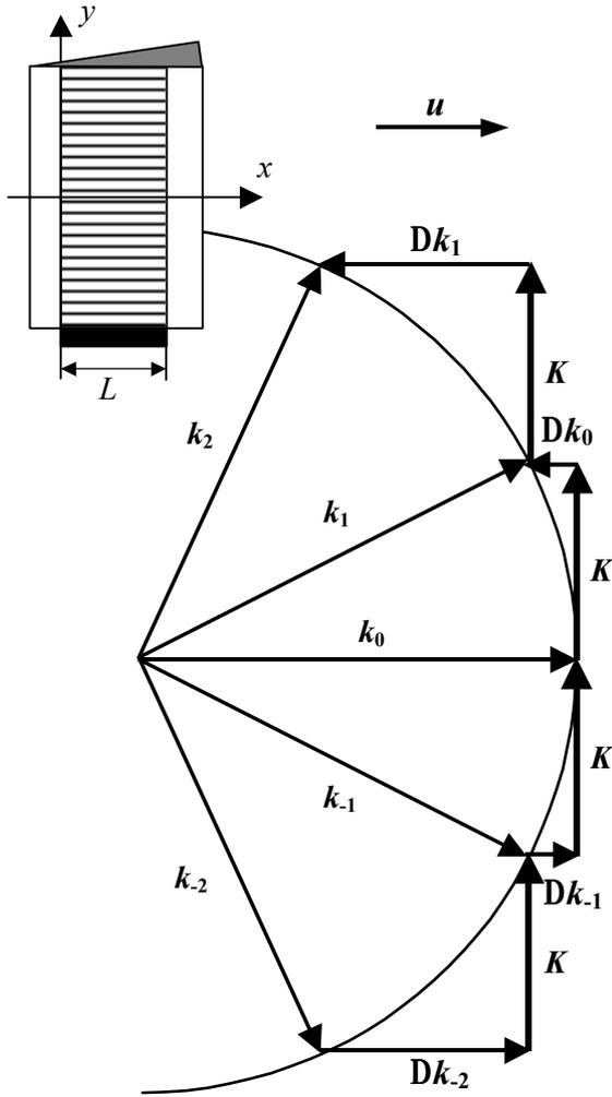
Figure 1: Set-up and wave vector diagram of AO-interaction in an isotropic medium.
