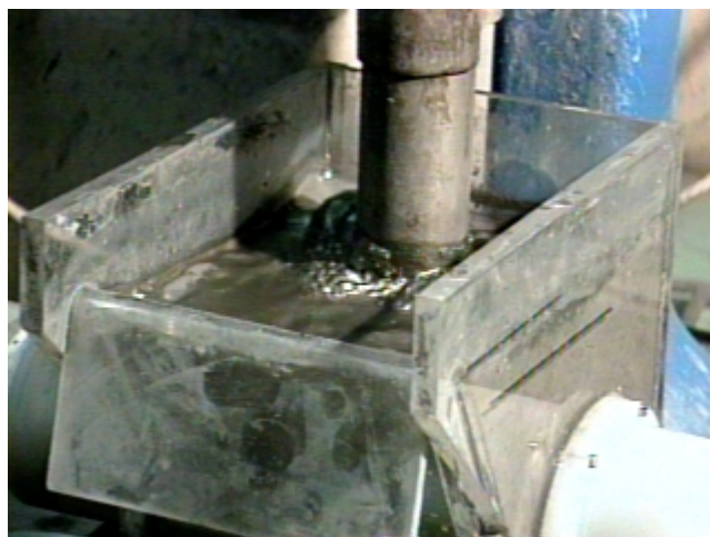
Fig. 1 Denver Cell for flotation experiments
