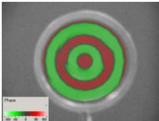
Fig. 3 Results for the inside of the vibrating ring visualized by the present method: upper picture, amplitude; lower, phase.
