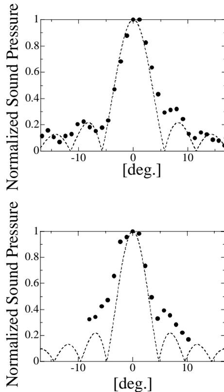
Fig. 12 Directivity in horizontal (upper) and vertical directions (lower).
