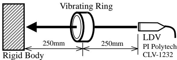
Fig. 2 Setup for measuring the standing wave field excited inside a vibrating ring.
