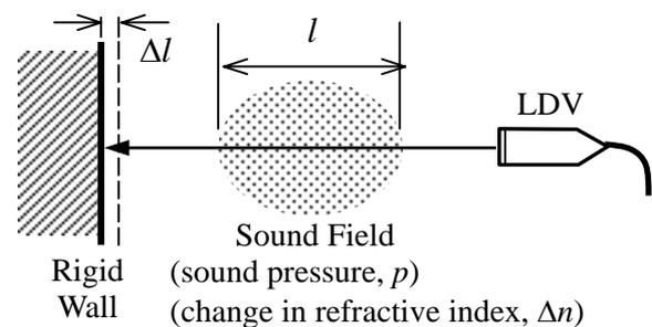
Fig. 1 Basic setup for sound pressure measurement by optical interferometry.
