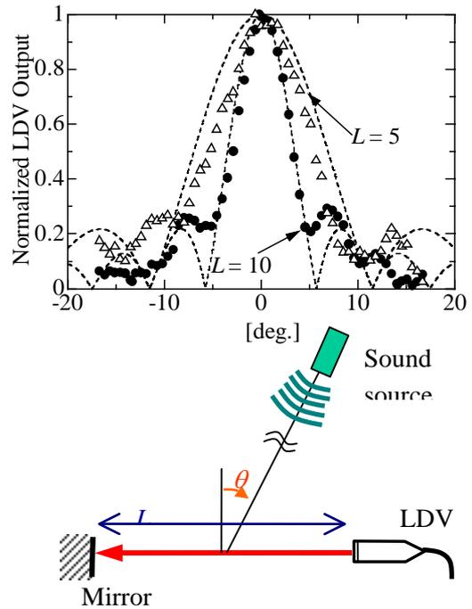
Fig. 8 Directivity in horizontal direction.
