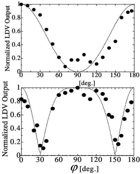
Fig. 10 Directivity patterns measured using the set-up of Fig. 9: upper figure shows the results in the case that  $d$  is equal to half a wavelength of the sound, while lower is the results when  $d$  is equal to the wavelength.
