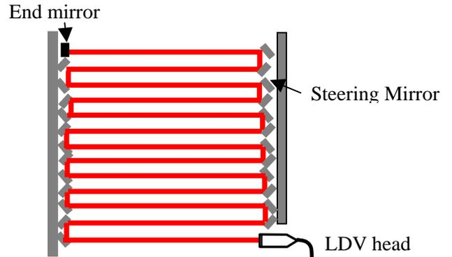
Fig. 11 Set-up for pencil beam.
