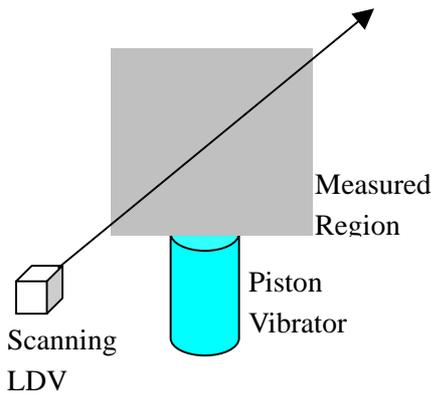
Fig. 5 Measured region for radiation field of a piston vibrator.
