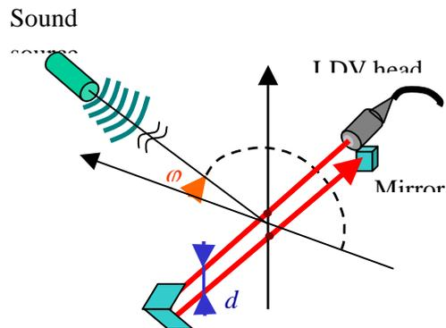
Fig. 9 Experimental setup for the directivity measurements in the plane vertical to the laser beams.
