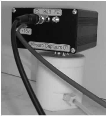
Fig.5 Compact package of the electronics directly connected atop the reaction chamber. The set-up directly includes frequency mixing and delivers either the signal of each resonator or the mixed signal.
