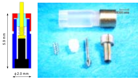
Fig. 12 Structure of the micro ultrasonic motor using cylindrical bulk transducer and its parts
