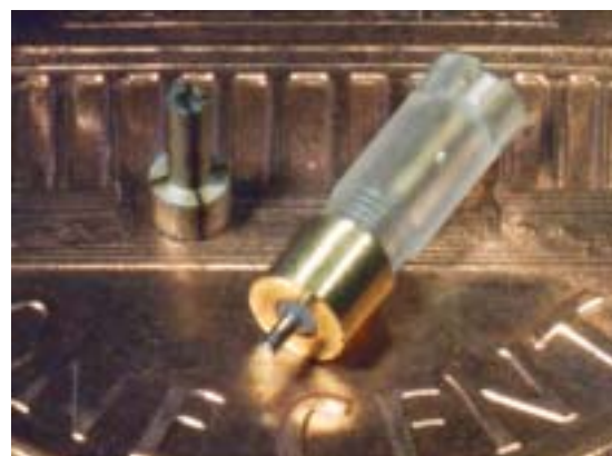
Fig. 13 Photograph of the micro ultrasonic motor (right) and piezoelectric vibrator (left) on US one cent coin
