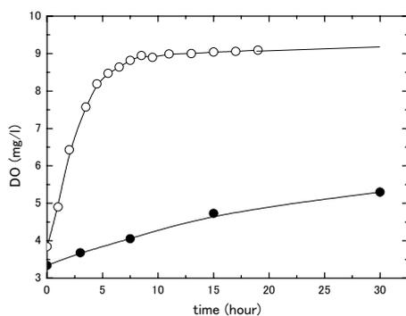
Figure.2 Time dependence of concentration of dissolved oxygen. (○): open system and (●) quasi-closed system.
