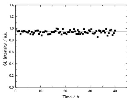
Figure.3 Time dependence of the SBSL intensity for 40 h.
