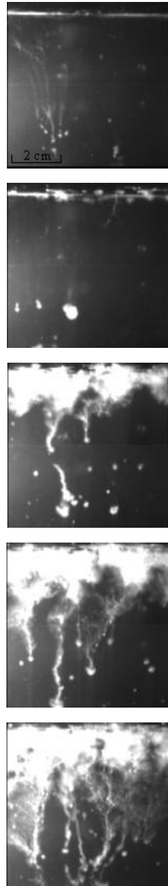
Figure 7: How CBS builds up when power is turned on (scattered light). Time increases from top to bottom. Length of sequence: 1.47 s.
