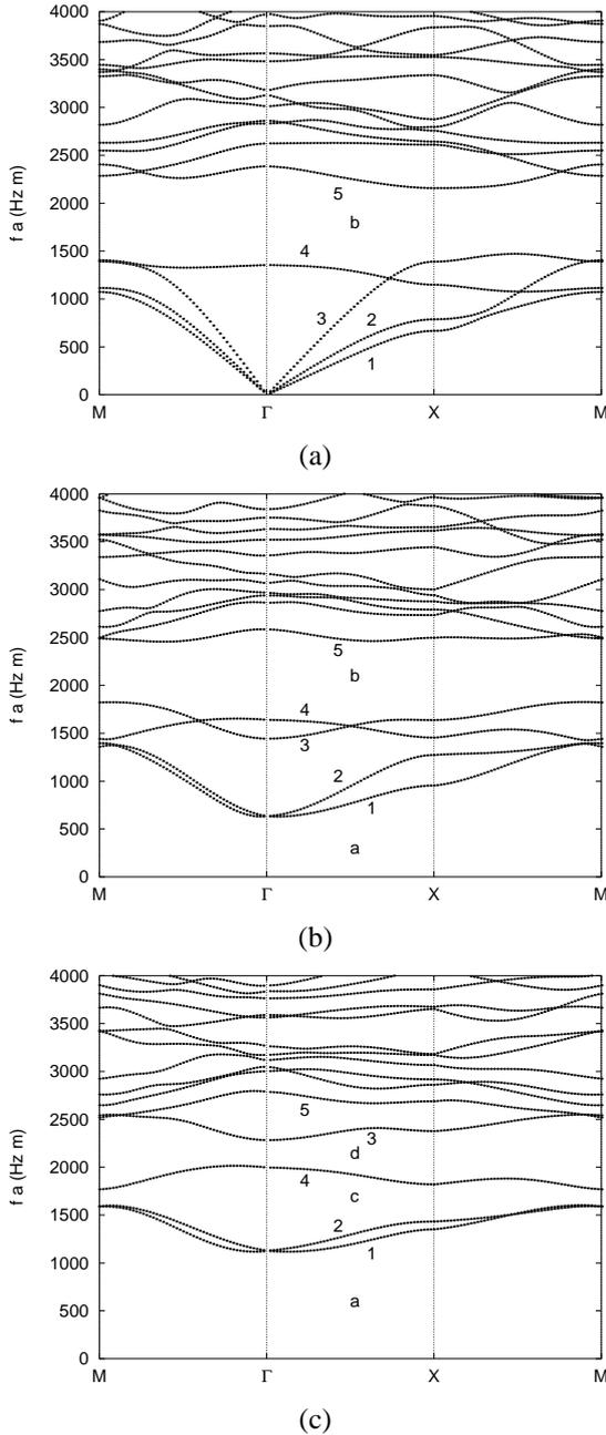
Figure 3: Dispersion curves along the  $M - \Gamma - X - M$  path shown in Fig. 1b, for (a)  $\gamma_z = 0$ , (b)  $\gamma_z = 0.25$ , and (c)  $\gamma_z = 0.4$ . The first five branches are numbered in the order of their appearance in the  $\gamma_z = 0$  dispersion diagram.
