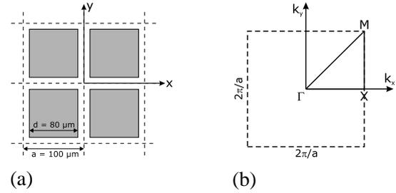
Figure 1: (a) Cross-section of a bi-periodic solid-solid phononic band-gap material, consisting of quartz rods in epoxy. (b) First Brillouin zone in the  $(k_x, k_y)$  plane.
