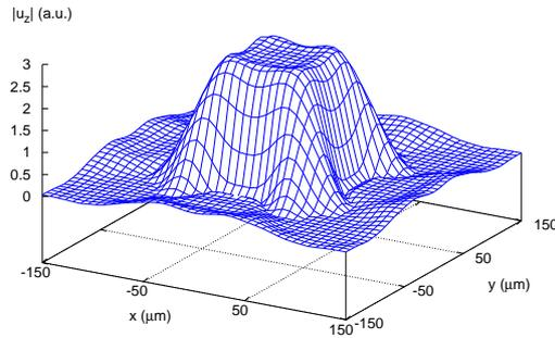
Figure 5: Relative magnitude of displacements of the tungsten/epoxy/AlN structure along the  $z$ -axis, for  $k_x = k_y = 0$ ,  $\gamma_z = 0.1$ , and  $f a = 848.2$  Hz m.
