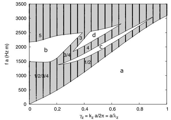
Figure 2: Projection of the phononic band structures in the  $(k_x, k_y)$  plane onto the  $(k_z, f)$  plane. Numbers indicate the positions of particular branches labeled in Fig. 3. Delimited white regions indicate absolute stop-bands in the  $(k_x, k_y)$  plane.
