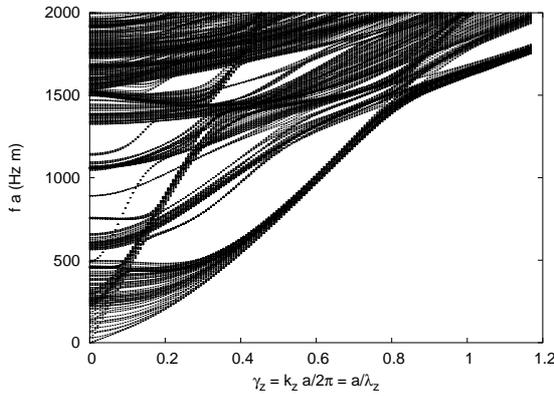
Figure 4: Projection of the phononic band structures in the  $(k_x, k_y)$  plane onto the  $(k_z, f)$  plane, for the tungsten/epoxy/AlN structure. Delimited white regions indicate absolute stop-bands in the  $(k_x, k_y)$  plane. Defect modes appear in these regions.
