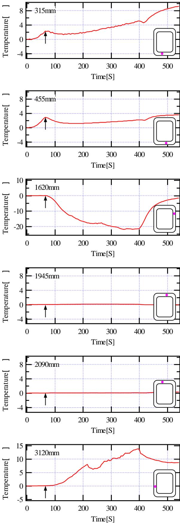
Fig. 3 Temperature variation in the loop-tube filled with the mixture of air and helium gas.
