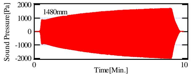
Fig. 5 Observed waveform in the loop-tube filled with air at 1480mm.
