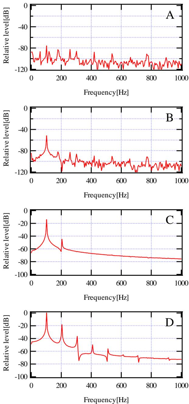
Fig. 7 Change of observed spectrum at 1480mm from heater in the loop-tube filled with air.
