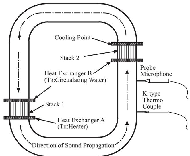
Fig. 1 Block diagram of measurement system for sound pressure and temperature variation.
