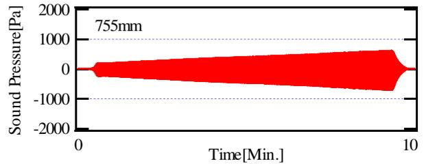
Fig. 4 Observed waveform in the loop-tube filled with air at 755mm.
