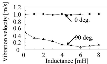
Figure 11: Vibration velocity vs. the inductance.
