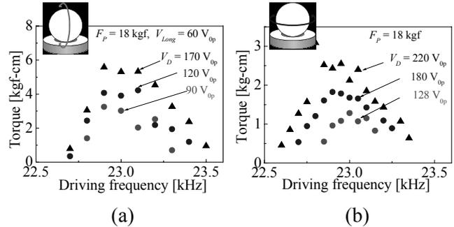
Figure 7: Torque characteristics: (a),  $x$  or  $y$ -axis; (b),  $z$ -axis.
