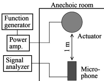
Figure 5: Sound pressure level measuring system.
