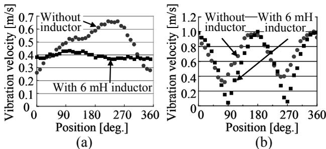
Figure 12: Vibration velocity vs. the angular position: (a), longitudinal vibration; (b), bending vibration.
