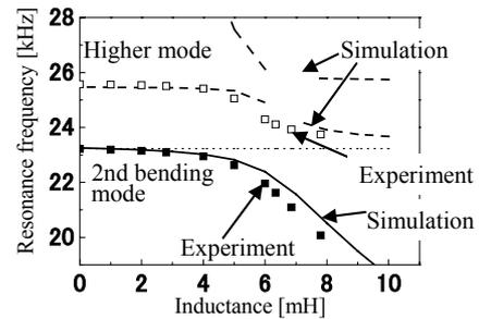
Figure 8: Resonance frequencies vs. the inductance.
