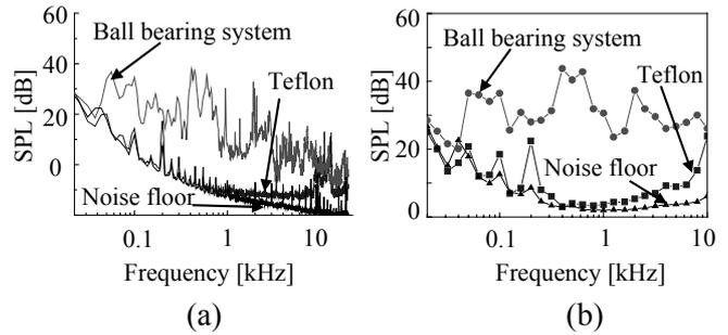
Figure 6: Frequency characteristics of sound pressure level measured for the different support mechanisms: (a), FFT analysis; (b), 1/3oct. band analysis.
