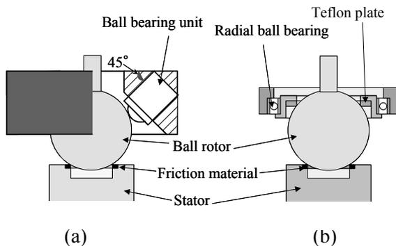
Figure 3: Support mechanism using: (a), three ball bearing units; (b), a Teflon plate.
