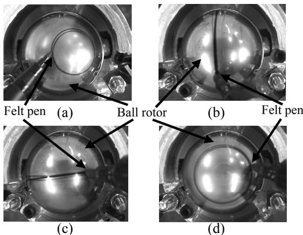
Figure 13: Pictures of the ball rotor orbit: (a), about the  $y$ -axis with coupling; (b), about the  $y$ -axis; (c),  $x$ -axis; (d),  $z$ -axis.
