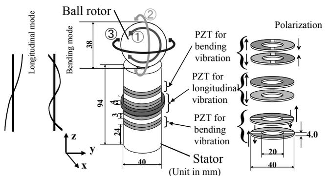
Figure 1: Motor configuration and the ball rotor rotation.
