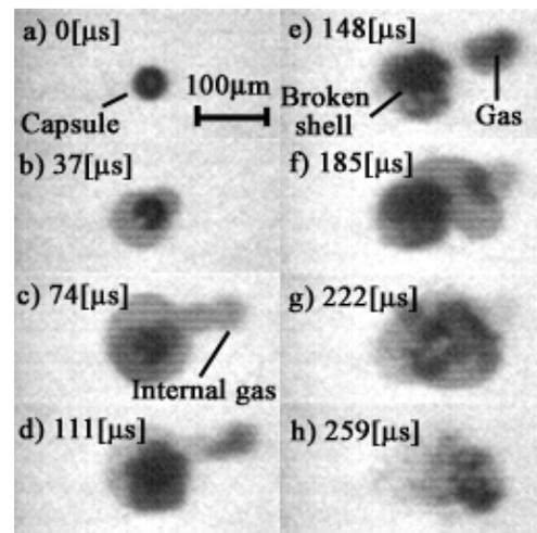
Figure 3 : Images of destruction of a single microcapsule. (f=115[kPa], P=100[kPa], R<sub>0</sub>=25[ $\mu\text{m}$ ], 27000[frames/sec])
