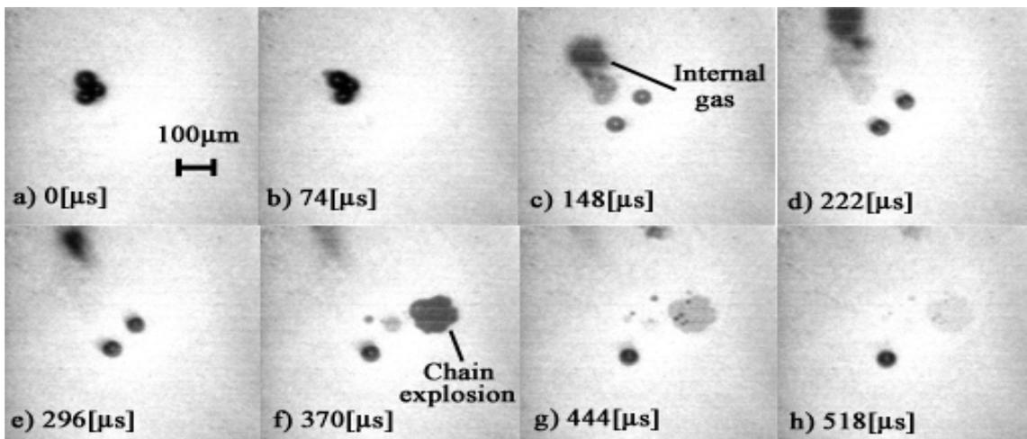
Figure 7 : Images of destruction of multi-capsules.(f=115[kHz], 13500[frames/sec])
