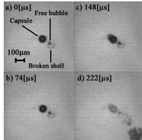
Figure 6 : Images of destruction of a capsule caused by a free bubble. (f=115[kHz], 13500[frames/sec])
