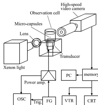
Figure 1 : Measurement system with a high-speed video camera.
