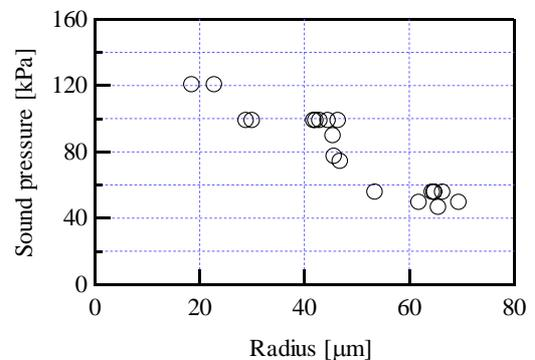
Figure 4 : Relationship between capsule radius and threshold sound pressure for capsule destruction.(f=115[kHz])
