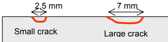
Figure 3. Schematic of cracks
