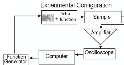
Figure 1: Experimental configuration for pure-tone S3D.
