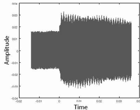
(clearly seen by the amplitude change in bottom figure), and post impact. Note the signal due to the impact and the associated ringing. The ringing dissipates but the amplitude change remains due to SD (not indefinitely: the material returns to its original state after some time). The probe frequency is located on the right-hand side of the modal peak as illustrated in Figure 2, and this is why the probe-wave amplitude decreases with the disturbance, in contrast to the next example.
