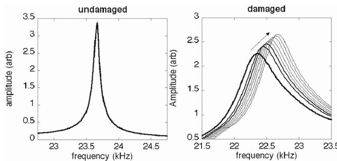
successive recovery. The sample recovery time shown is 141 seconds. Full recovery took approximately one hour. Clearly it is only necessary to look at one or two probe sweeps to discern whether or not the sample is damaged so the method can be applied relatively quickly. In this case, one has both the frequency and amplitude. However, tracking initial frequency shift during fast dynamics and the recovery of a modal peak is extremely robust.
