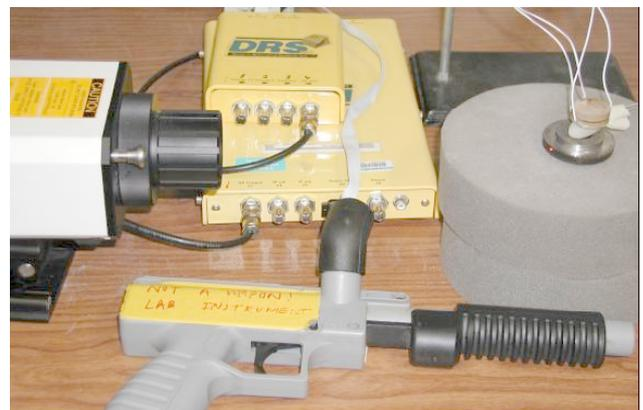
was used to couple the ceramic, probe wave source from the sample. An airgun was used to induce elastic nonlinear response. The probe-wave frequency-sweep was accomplished using the resonant ultrasound spectroscopy device manufactured by DRS., Inc. A Polytech laser vibrometer was used to detect the signal. Independent of the S3D method, the non-contact sources developed here are extremely useful and could be applied to
