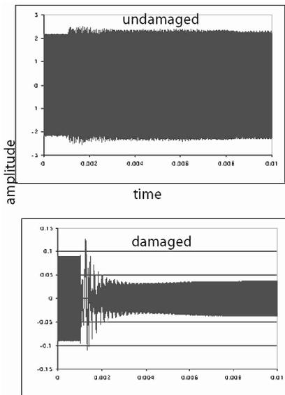
Figure 3. The slope amplifier at work. The x-axis is time, and the y-axis is amplitude. The damaged sample is easily identified due to the significant amplitude change. The method can be quickly applied because all that is required is to view whether or not an amplitude change takes place.
