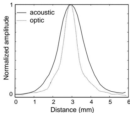
Figure 3: Amplitude profiles measured in the focal plane of a 2.25-MHz frequency transducer ( $f$ -number  $\approx 1$ ) with the ultrasonic and optical probes.
