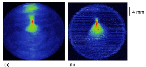
Figure 5: C-scan images of the velocity measured on the P plane, with the ultrasonic (a) and optical (b) probes.
