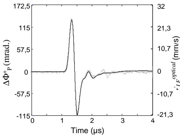
Figure 2: Phase modulation  $\Delta\Phi_p^+$  detected with the ultrasonic probe (thick line), when the LF motion is generated by a 2.5-MHz planar transducer (diameter: 25.4 mm). This result is compared with the particle velocity  $v_{LF}^{optical}$  (dashed line) derived from the optical measurement of the displacement. The acoustic measurement has been shifted by a quantity equal to the travel time  $L/c_0$  between the vibrating surface and the probe transducer.
