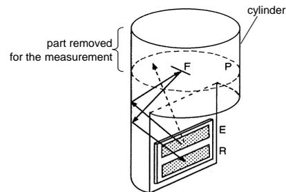
Figure 4: Industrial part tested by a dual transducer. The region highlighted for the non-destructive test is determined by probing the surface denoted P. Dashed arrow shows the direct acoustic path from the emitter E to the P plane.
