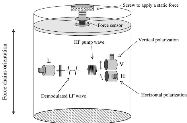
Figure 1: Scheme of the experiment. The propagation direction is orthogonal to the force chains preferential orientation. Propagation distance is  $16cm$ .
