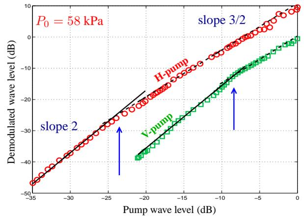
Figure 3: Demodulated signal amplitude dynamics as a function of the pump strain level. The pump wave frequency is  $80kHz$  and the demodulated wave frequency is  $5kHz$ .
