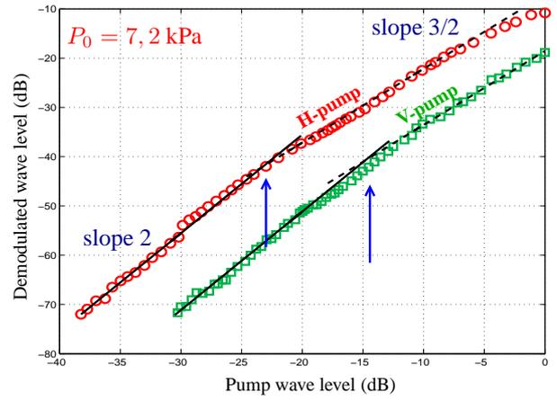
Figure 2: Demodulated signal amplitude dynamics as a function of the pump strain level. The pump wave frequency is  $80kHz$  and the demodulated wave frequency is  $5kHz$ .
