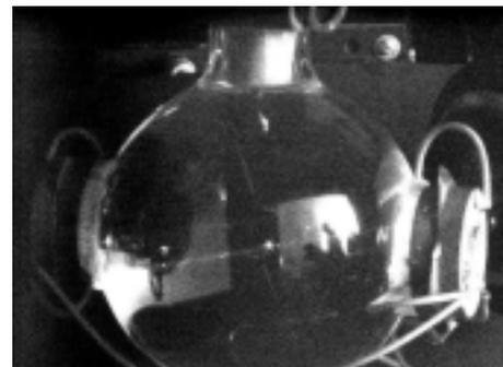
Figure 9 Photo of the resonant flask
